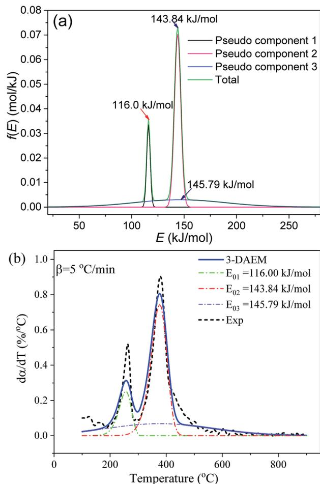
Fig. 8 Gaussian  $f(E)$  and  $d\alpha/dT$  of the pseudo components calculated by 3-DAEM during the thermal debinding process at a heating rate of  $5\text{ }^{\circ}\text{C min}^{-1}$ : (a)  $f(E)$  and (b)  $d\alpha/dT$ .
