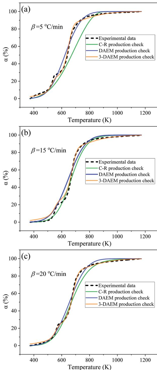
Fig. 9 Comparison between experimental and model calculated conversion rates ( $\alpha$ ) obtained with the three different models: (a)  $5\text{ }^{\circ}\text{C min}^{-1}$ , (b)  $15\text{ }^{\circ}\text{C min}^{-1}$  and (c)  $20\text{ }^{\circ}\text{C min}^{-1}$ .
