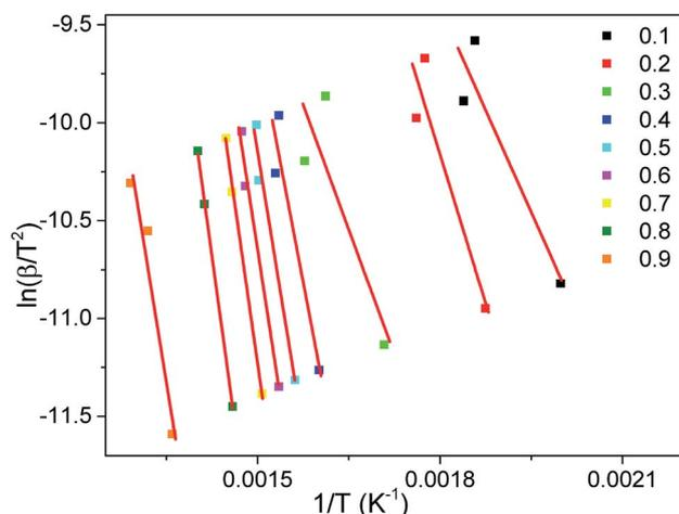
Fig. 5 Arrhenius plot of  $\ln(\beta/T^2)$  vs.  $1/T$  at the different conversion rates.
