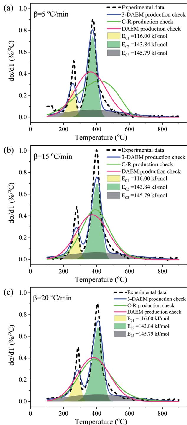
Fig. 10 Comparison between experimental and model calculated reaction rates ( $d\alpha/dT$ ) obtained with the three different models: (a)  $5 \text{ °C min}^{-1}$ , (b)  $15 \text{ °C min}^{-1}$  and (c)  $20 \text{ °C min}^{-1}$ .
