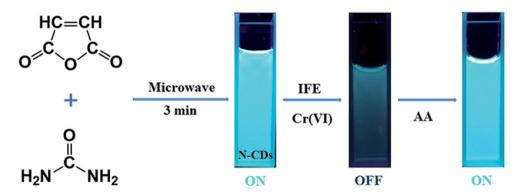
Fig. 1 Schematic of the synthesis of the N-doped CDs (N-CDs) and the on-off-on detection of chromium(v) [Cr(vi)] and ascorbic acid (AA) based on the inner filter effect (IFE). The fluorescence images were obtained under 365 nm UV light. ON: fluorescent N-CDs and OFF: quenched N-CDs.
