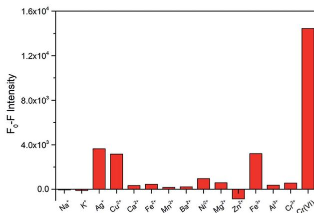
Fig. 5 Fluorescence intensity changes of the N-CDs for various metal ions in water. The concentrations of all the metal ions were 50 μM.  $F_0$  and  $F$  are the fluorescence intensities of the N-CDs without and with the addition of metal ions.
