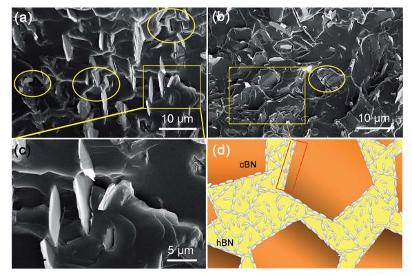
Fig. 7 SEM images of the cross-sectional morphology for h-BN/c-BN/EP composites containing h-BN/c-BN hybrid fillers of 3:4 (a) and 2:1(b). (c) Magnification of the selected rectangular region in (a). (d) Schematic representations for ideal model structures for h-BN/c-BN hybrid fillers arranged within the EP matrix.
