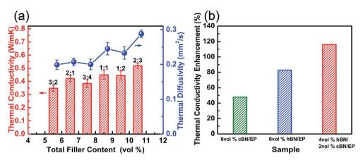
Fig. 5 (a) Thermal conductivity and thermal diffusivity of the h-BN/c-BN/EP composites at different total filler content. (b) At 6 vol% total filler loading, thermal conductivity enhancement of c-BN/EP, h-BN/EP and h-BN/c-BN/EP composites, respectively.
