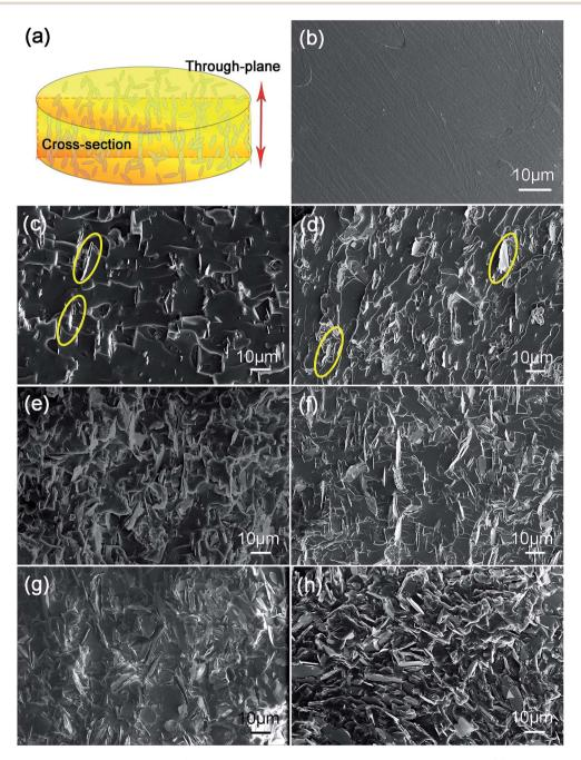
Fig. 3 (a) Schematic illustration of the composites. SEM images of cross-sectional morphology of the neat EP (b) and EP composites containing 3 vol% (c), 6 vol% (e), and 9 vol% (g) pristine h-BN and 3 vol% (d), 6 vol% (f) and 9 vol% (h) modified h-BN comparably.
