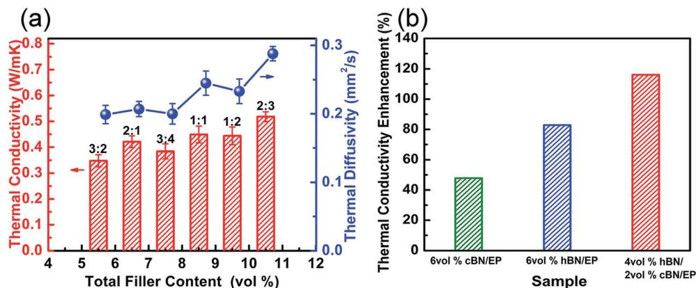
Fig. 5 (a) Thermal conductivity and thermal diffusivity of the h-BN/c-BN/EP composites at different total filler content. (b) At 6 vol% total filler loading, thermal conductivity enhancement of c-BN/EP, h-BN/EP and h-BN/c-BN/EP composites, respectively.
