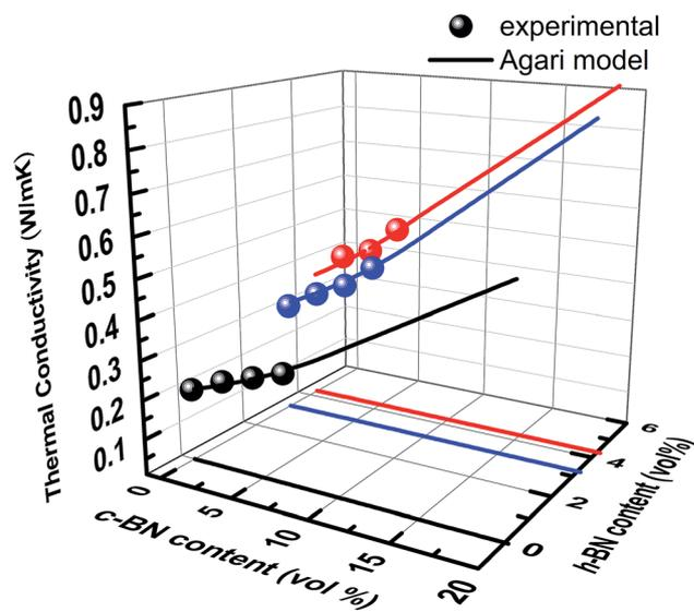
Fig. 6 Thermal conductivity of hybrid fillers h-BN/c-BN and sole filler of c-BN in EP composites as function of h-BN and c-BN loading content, respectively. The solid lines are theoretical predications based on Agari's model.
