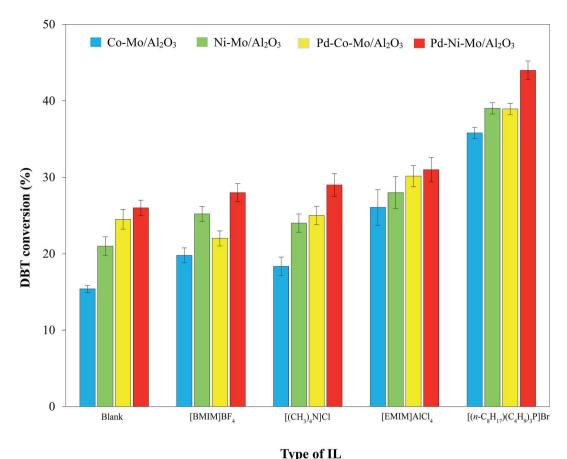
Fig. 7 Comparison of DBT conversion by different catalysts (0.1 g) combined with 4 g of each IL at  $160 \,^{\circ}$ C, 3 MPa H<sub>2</sub> pressure and 4 h reaction time using 30 mL of 1000 ppm DBT solution.
