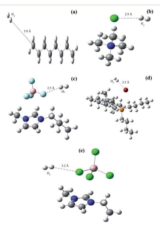
Fig. 8 DFT simulation indicating interaction of  $H_2$  with (a) n-octane, (b) [(CH<sub>3</sub>)<sub>4</sub>N]Cl, (c) [BMIM]BF<sub>4</sub>, (d) [(n-C<sub>8</sub>H<sub>17</sub>)(C<sub>4</sub>H<sub>9</sub>)<sub>3</sub>P]Br and (e) [EMIM]AlCl<sub>4</sub> in terms of binding energy and relative distance between atoms.
