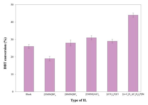
Fig. 6 Comparison of DBT conversion by Pd-Ni-Mo/Al<sub>2</sub>O<sub>3</sub> (0.1 g) combined with 4 g of each IL at 160 °C, 3 MPa H<sub>2</sub> pressure, and 4 h reaction time with 30 mL of 1000 ppm DBT solution.
