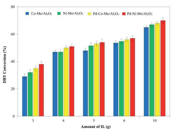
Fig. 12 Effect of amount of IL on DBT conversion using 30 mL of 1000 ppm DBT solution, 1 MPa  $H_2$  pressure, 120 °C reaction temperature, 200 rpm stirring speed and 4 h reaction time.
