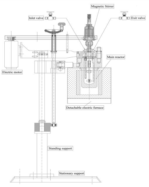
Fig. 1 Design of the batch autoclave reactor.
