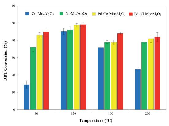
Fig. 10 Effect of reaction temperature on DBT conversion utilizing 0.1 g of each catalyst at 3 MPa  $H_2$  pressure, 4 h reaction time, 200 rpm stirring speed, 30 mL of 1000 ppm DBT solution and 4 g of  $[(n-C_8H_{17})(C_4H_9)_3P]Br$ .
