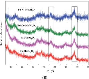
Fig. 3 XRD patterns of (A) support and fresh catalysts and (B) spent catalysts.
