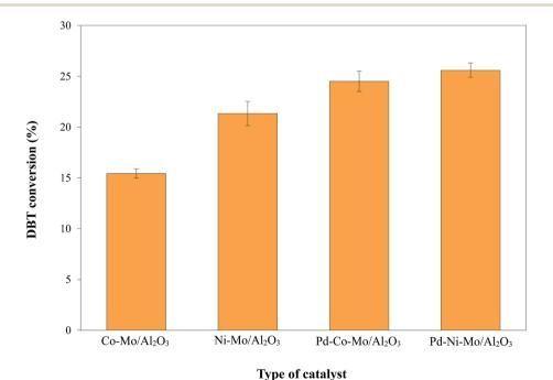
Fig. 5 DBT conversion by 0.1 g of presulfided catalyst at 3 MPa H<sub>2</sub> pressure, 160 °C and 4 h reaction time using 30 mL of 1000 ppm DBT solution.
