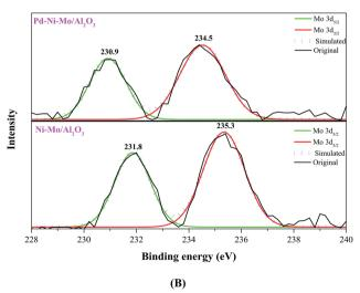
Fig. 4 High-resolution XPS spectra of Mo 3d (A)  $Co-Mo/Al_2O_3$  and  $Pd-Co-Mo/Al_2O_3$  and (B)  $Ni-Mo/Al_2O_3$  and  $Pd-Ni-Mo/Al_2O_3$  catalysts.
