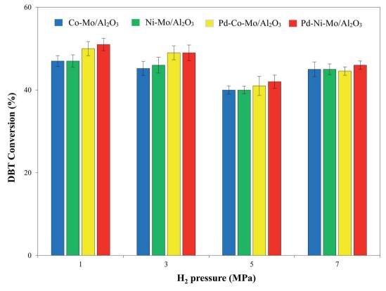
Fig. 11 Effect of  $H_2$  pressure on the HDS activity of different catalysts (0.1 g each) in the presence of 4 g of  $[(n-C_8H_{17})(C_4H_9)_3P]$ Br at 120 °C and 4 h reaction time and 30 mL of 1000 ppm DBT solution.
