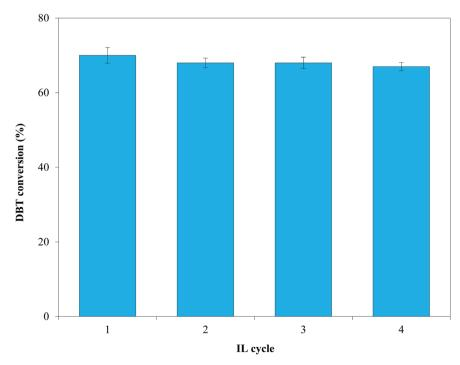
Fig. 13 Effect of four consecutive recycles on DBT conversion using 10 g of  $[(n-C_8H_{17})(C_3H_7)_3P]$ Br coupled with 0.1 g of Pd-Ni-Mo/Al<sub>2</sub>O<sub>3</sub> catalyst at 1 MPa H<sub>2</sub> pressure, 120 °C temperature, 4 h reaction time, 200 rpm stirring speed and 30 mL of 1000 ppm DBT solution.
