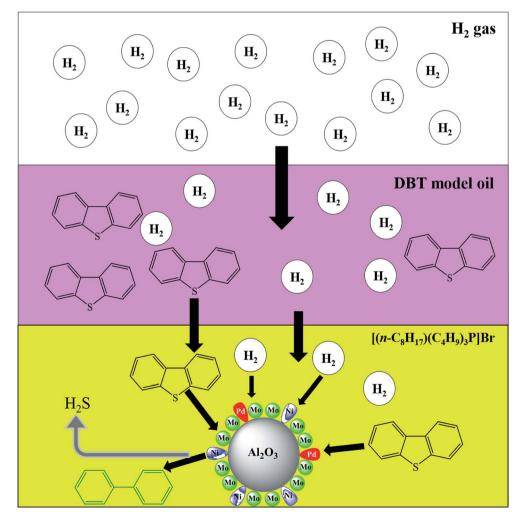
Fig. 9 HDS of DBT process demonstrating transport of H<sub>2</sub> through oil and IL phase reaching the solid catalyst surface.
