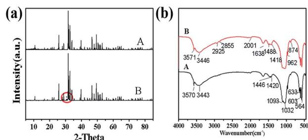
Fig. 9 XRD patterns and FTIR spectrum of (a) HAP<sup>M-H</sup>, (b) HAP<sup>H</sup>.
