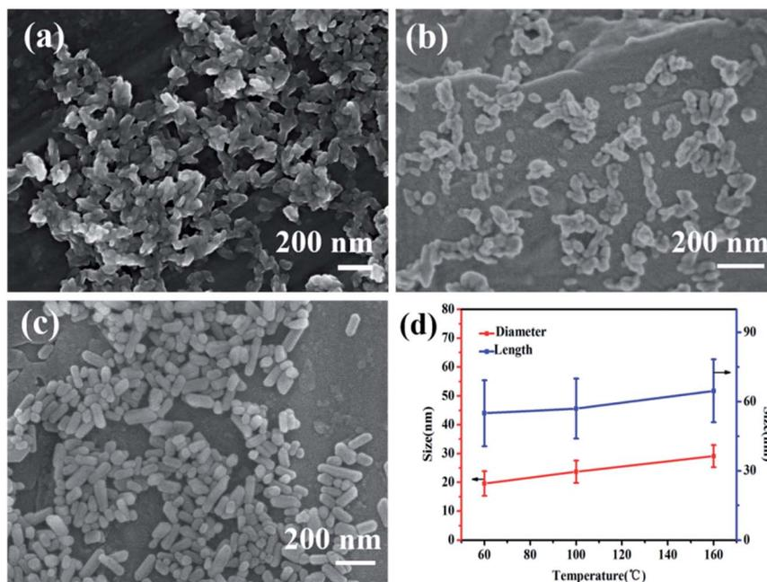
Fig. 2 SEM images of nano-HAP<sup>M-H</sup> samples obtained at (a) 60 °C for 40 minutes, (b) 100 °C for 40 minutes, (c) 160 °C for 40 minutes, and (d) the size of samples obtained at different reaction temperature.
