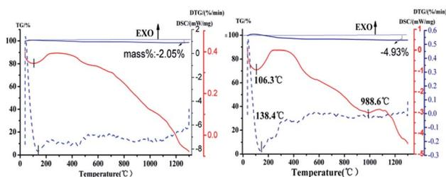
Fig. 8 TG-DSC thermogram of (a) HAP<sup>M-H</sup>, (b) HAP<sup>H</sup>.
