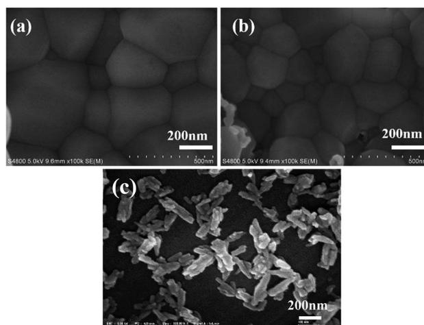
Fig. 11 SEM images of (a) nano-HAP<sup>H</sup> ceramics, (b) nano-HAP<sup>M-H</sup> ceramics, (c) nano-HAP<sup>H</sup> powder.
