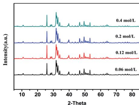
Fig. 5 XRD patterns of HAP with different reaction concentration of  $\text{Na}_2\text{HPO}_4$ .
