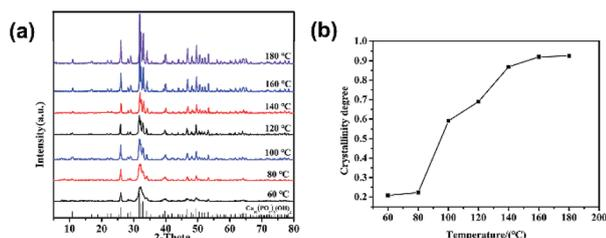
Fig. 1 (a) XRD patterns and (b) crystallinity of HAP with different reaction temperatures.
