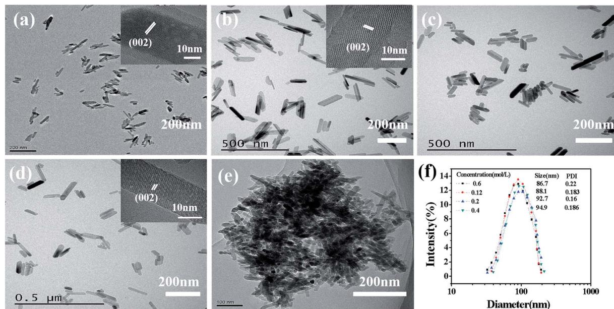
Fig. 6 TEM images of samples with different concentration of  $\text{Na}_2\text{HPO}_4$  (a)  $0.06 \text{ mol L}^{-1}$ , (b)  $0.12 \text{ mol L}^{-1}$ , (c)  $0.2 \text{ mol L}^{-1}$ , (d)  $0.4 \text{ mol L}^{-1}$ , (e)  $0.5 \text{ mol L}^{-1}$  synthesized by M-H method and (f) size distribution of samples with different  $\text{Na}_2\text{HPO}_4$  concentration.
