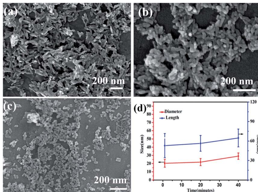
Fig. 4 SEM images of nano-HAP<sup>M-H</sup> obtained at (a) 160 °C for 1 minute, (b) 160 °C for 20 minutes, (c) 160 °C for 40 minutes, and (d) the size of samples obtained at different time.
