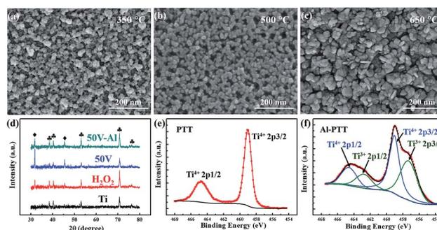
Fig. 2 Typical FE-SEM images of PTT-50 reduced at (a) 350 °C, (b) 500 °C, (c) 650 °C. (d) X-ray diffraction patterns of Ti plates before and after different treatment (◆: anatase TiO<sub>2</sub>, ♣: Ti). Ti 2p XPS spectra of (e) PTT-50 and (f) Al-PTT-50.
