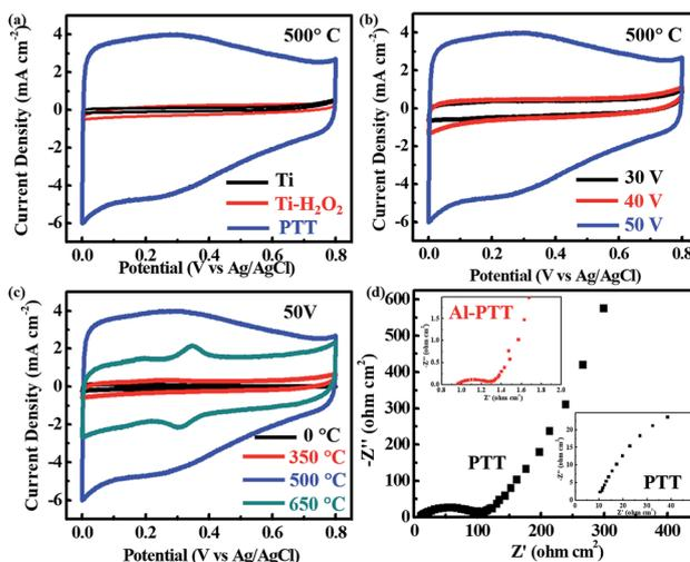
Fig. 3 CV curves of electrodes reduced at 500 °C at the scan rate of 50 mV s<sup>-1</sup>: (a) raw Ti, Ti-H<sub>2</sub>O<sub>2</sub>, PTT-50; (b) raw Ti, PTT-30, PTT-40, PTT-50. (c) PTT-50 reduced at different temperatures ranging from 0 to 650 °C. (d) Nyquist plots of PTT-50 and Al-PTT-50, insets are enlargements of the high frequency regions.
