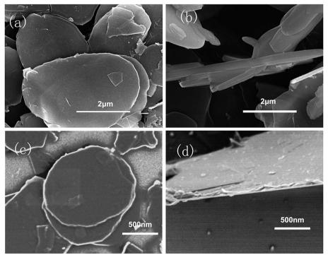
Fig. 4 SEM images of h-BN and MBN (a) lateral size of h-BN,  $3-5 \mu m$ ; (b) thickness of h-BN, 300 nm; (c) lateral size of MBN,  $1-2 \mu m$ ; (d) thickness of MBN, 30 nm.
