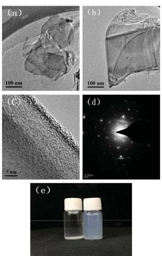
Fig. 5 TEM images of MBN (a)  $\vartheta$  (b) low resolution; (c) HRTEM; (d) electron diffraction pattern; and (e) photos of h-BN and MBN dispersed in ethanol solvent for 24 h.
