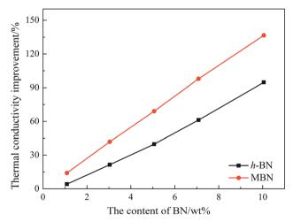
Fig. 10 Thermal conductivity improvement of EP/PBMG/BN composites with different BN contents.
