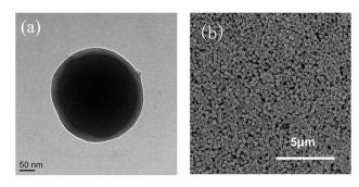
Fig. 3 PBMG latex (a) TEM core-shell structure; (b) SEM particle distribution.
