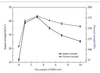
Fig. 8 Impact and flexural strengths of epoxy composites with various MBN contents.
