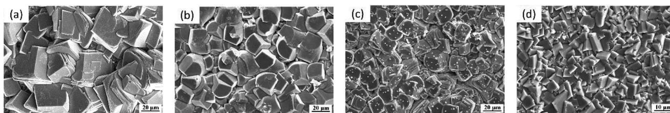
Fig. 3 Surface morphologies of N80 steel under various  $\text{CO}_2$  partial pressures at  $100\text{ }^\circ\text{C}$ : (a) 0.15 MPa; (b) 0.6 MPa; (c) 1 MPa; and (d) 4 MPa.
