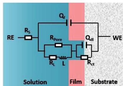
Fig. 6 Electrochemical equivalent circuit used for EIS fittings.
