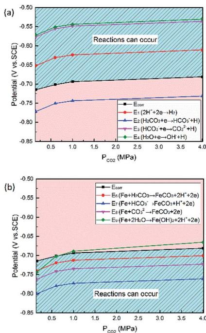
Fig. 8 Comparison of the measured corrosion potential ( $E_{\text{corr}}$ ) and the calculated equilibrium potential of anodic (a) and cathodic (b) reactions as a function of the  $\text{CO}_2$  partial pressure.
