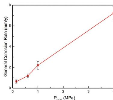
**Fig. 2** Corrosion rate of N80 carbon steel at various CO<sub>2</sub> partial pressures and 100 °C.
