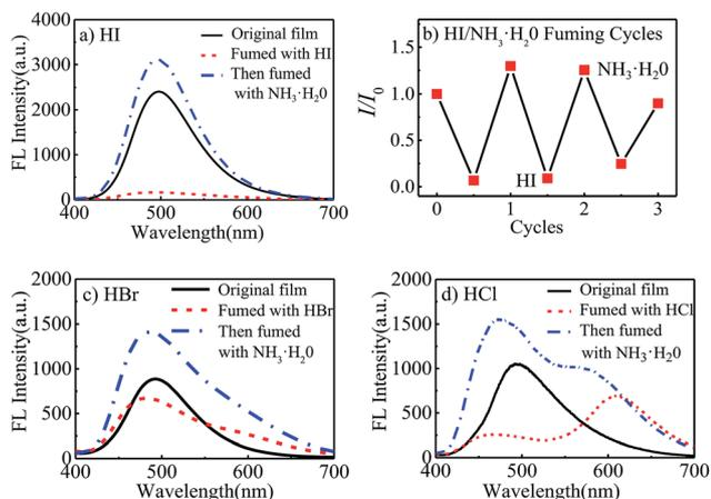
**Fig. 3** (a) Fluorescence emission spectra of STMPU-50 film before and after fumed with hydroiodic acid and then fumed with  $\text{NH}_3 \cdot \text{H}_2\text{O}$ ; (b) the quenching and recovery test by  $\text{HI-NH}_3 \cdot \text{H}_2\text{O}$  fuming cycles; fluorescence emission spectra of STMPU-50 film before and after fumed with (c) hydrobromic acid and (d) hydrochloric acid, and then fumed with  $\text{NH}_3 \cdot \text{H}_2\text{O}$ .
