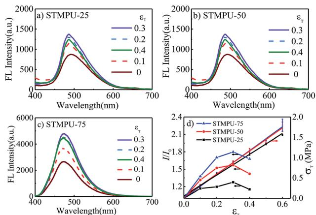
**Fig. 2** Fluorescence emission spectra of (a) STMPU-25, (b) STMPU-50 and (c) STMPU-75 films at different tensile strains; (d) true stress–strain curves and fluorescence peak intensity–true strain curves of three AEE polyurethanes.
