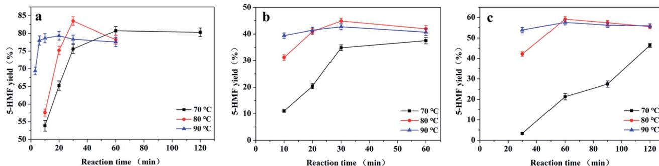
Fig. 4 Effect of the reaction temperature on the yield of 5-HMF from fructose (a), sucrose (b), and inulin (c). Reaction conditions: catalyst (50 mg), [BMIM][Cl] (2.50 g), fructose (0.50 g), sucrose (0.25 g), and inulin (0.25 g).
