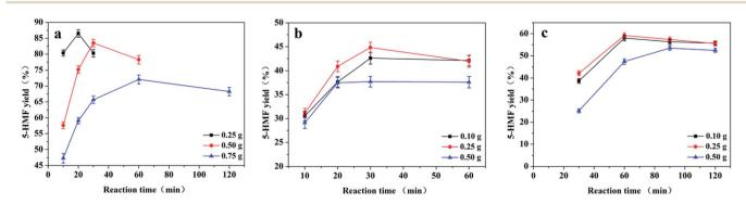
Fig. 6 Effect of the substrate loading on the yield of 5-HMF from fructose (a), sucrose (b), and inulin (c). Reaction conditions: catalyst (50 mg), [BMIM][CI] (2.50 g), and reaction temperature (80 °C).
