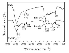
Fig. 3 FTIR spectra of the CMs and CM-SO<sub>3</sub>H
