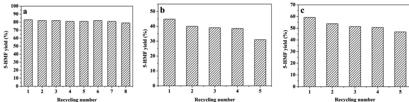
Fig. 7 Reusability of CM-SO<sub>3</sub>H for fructose (a), sucrose (b), and inulin (c) conversion to 5-HMF. Reaction conditions: fructose (0.50 g), sucrose (0.25 g), or inulin (0.25 g); CM-SO<sub>3</sub>H (50 mg); [BMIM][Cl] (2.50 g); temperature (80 °C); and reaction time (30 min).
