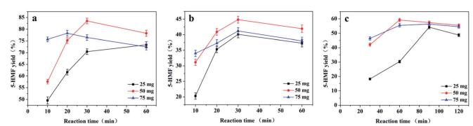
Fig. 5 Effect of catalyst loading on the yield of 5-HMF from fructose (a), sucrose (b), and inulin (c). Reaction conditions: [BMIM][Cl] (2.50 g), fructose (0.50 g), sucrose (0.25 g), inulin (0.25 g), and reaction temperature (80 °C).
