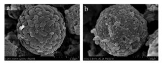
Fig. 2 SEM images of CMs (a) and CM-SO<sub>3</sub>H (b).
