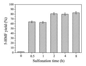
Fig. 1 The effect of sulfonation time on the 5-HMF yield from fructose. Reaction conditions: fructose (0.50 g), catalyst (50 mg), [BMIM] [CI] (2.50 g), reaction temperature (80 °C), and reaction time (30 min).
