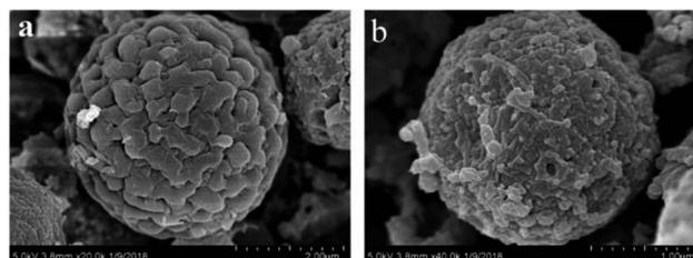
Fig. 2 SEM images of CMs (a) and CM-SO<sub>3</sub>H (b).
