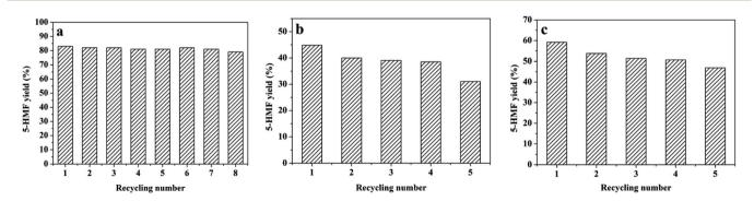
Fig. 7 Reusability of CM-SO<sub>3</sub>H for fructose (a), sucrose (b), and inulin (c) conversion to 5-HMF. Reaction conditions: fructose (0.50 g), sucrose (0.25 q), or inulin (0.25 q); CM-SO<sub>3</sub>H (50 mq); [BMIM][CI] (2.50 q); temperature (80 °C); and reaction time (30 min).
