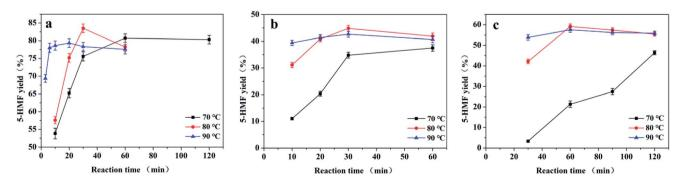
Fig. 4 Effect of the reaction temperature on the yield of 5-HMF from fructose (a), sucrose (b), and inulin (c). Reaction conditions: catalyst (50 mg), [BMIM][Cl] (2.50 g), fructose (0.50 g), sucrose (0.25 g), and inulin (0.25 g).
