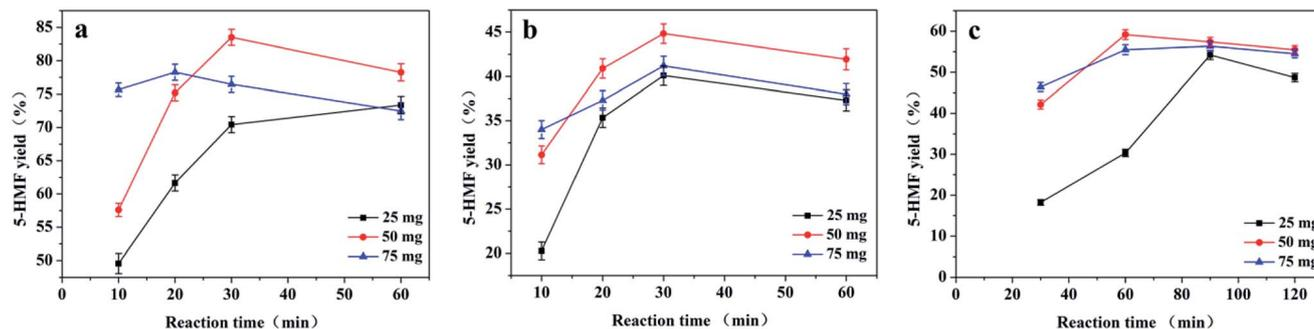
Fig. 5 Effect of catalyst loading on the yield of 5-HMF from fructose (a), sucrose (b), and inulin (c). Reaction conditions: [BMIM][Cl] (2.50 g), fructose (0.50 g), sucrose (0.25 g), inulin (0.25 g), and reaction temperature (80 °C).
