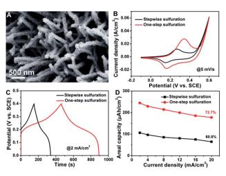
Fig. 7 (A) SEM image of NiCo<sub>2</sub>S<sub>4</sub>@NiCo<sub>2</sub>S<sub>4</sub> hybrid NTSAs synthesized by the stepwise sulfuration method, (B–D) comparison of the electrochemical properties for the NiCo<sub>2</sub>S<sub>4</sub>@NiCo<sub>2</sub>S<sub>4</sub> NTSAs obtained from different synthetic pathways: (B) CV curves, (C) GCD curves, and (D) rate capability.
