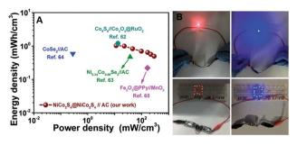
Fig. 9 (A) Ragone plot of the  $NiCo_2S_4$ @ $NiCo_2S_4$ //AC solid-state HSC device, as compared with that of some previously reported HSC devices in literature, (B) photographs of two assembled HSC devices connected in series, which can power 12 LEDs in red or blue simultaneously.
