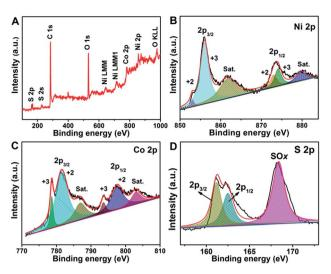
Fig. 4 XPS spectra of (A) survey, (B) Ni 2p, (C) Co 2p and (D) S 2p for the  $NiCo_2S_4@NiCo_2S_4$  hybrid NTSAs.
