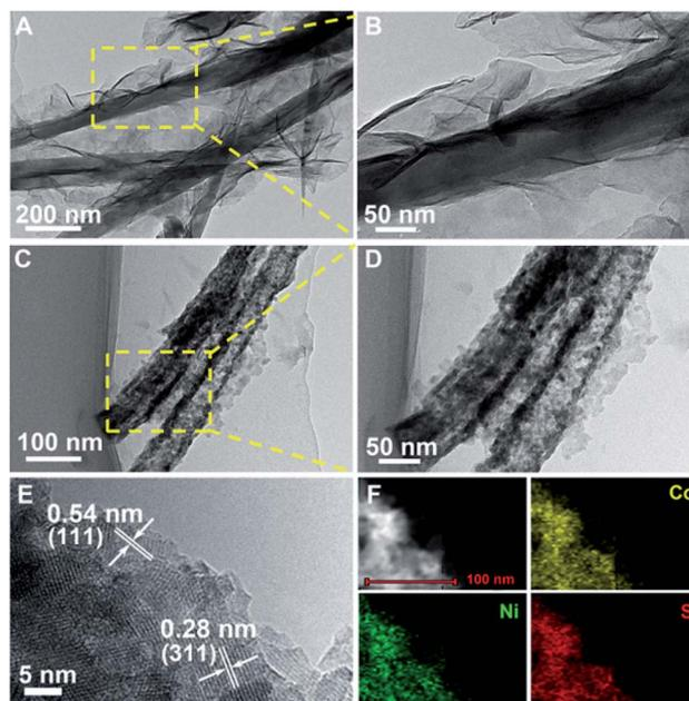
Fig. 3 Typical TEM images of (A and B) Ni–Co precursor@Ni–Co precursor NWSAs, and (C and D) NiCo<sub>2</sub>S<sub>4</sub>@NiCo<sub>2</sub>S<sub>4</sub> NTSAs at low- and high-magnifications, respectively; (E) HRTEM image of the NiCo<sub>2</sub>S<sub>4</sub>@NiCo<sub>2</sub>S<sub>4</sub> NTSAs near the surface part; (F) elemental mapping results of the NiCo<sub>2</sub>S<sub>4</sub>@NiCo<sub>2</sub>S<sub>4</sub> NTSAs.
