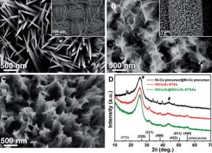
Fig. 2 (A–C) Typical SEM images: (A) Ni–Co precursor NWAs, (B) Ni–Co precursor@Ni–Co precursor NWSAs, and (C) NiCo $_2$ S $_4$ @NiCo $_2$ S $_4$  hybrid NTSAs. Inset shows the corresponding low-magnification SEM images. (D) XRD patterns of Ni–Co precursor@Ni–Co precursor NWSAs, NiCo $_2$ S $_4$  NTAs and NiCo $_2$ S $_4$ @NiCo $_2$ S $_4$  NTSAs. The peaks marked by "#" are arising from carbon cloth.
