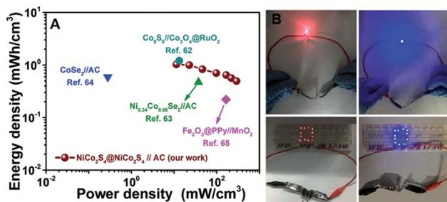
Fig. 9 (A) Ragone plot of the  $\text{NiCo}_2\text{S}_4@\text{NiCo}_2\text{S}_4//\text{AC}$  solid-state HSC device, as compared with that of some previously reported HSC devices in literature, (B) photographs of two assembled HSC devices connected in series, which can power 12 LEDs in red or blue simultaneously.
