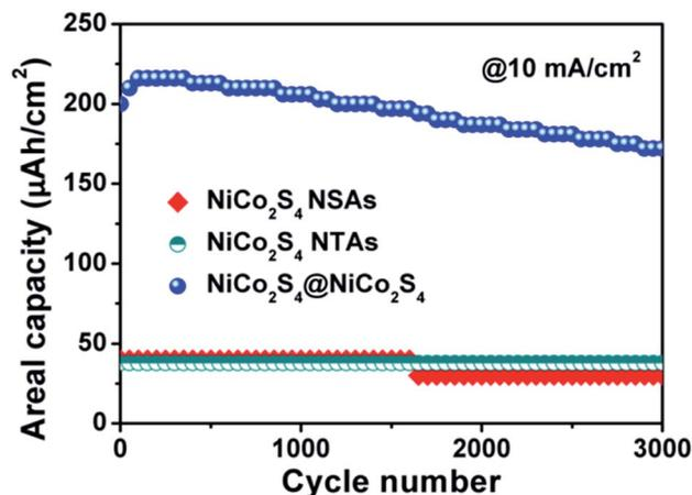
Fig. 6 Cycling stability for the electrodes of NiCo<sub>2</sub>S<sub>4</sub> NTAs, NiCo<sub>2</sub>S<sub>4</sub> NSAs and NiCo<sub>2</sub>S<sub>4</sub>@NiCo<sub>2</sub>S<sub>4</sub> NTASs at a current density of 10 mA cm<sup>-2</sup>.
