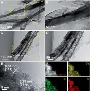
Fig. 3 Typical TEM images of (A and B) Ni–Co precursor@Ni–Co precursor NWSAs, and (C and D) NiCo $_2$ S $_4$ @NiCo $_2$ S $_4$  NTSAs at low- and high-magnifications, respectively; (E) HRTEM image of the NiCo $_2$ S $_4$ @NiCo $_2$ S $_4$  NTSAs near the surface part; (F) elemental mapping results of the NiCo $_2$ S $_4$ @NiCo $_2$ S $_4$
