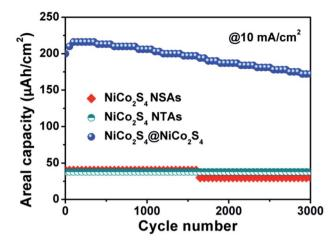
Fig. 6 Cycling stability for the electrodes of NiCo<sub>2</sub>S<sub>4</sub> NTAs, NiCo<sub>2</sub>S<sub>4</sub> NSAs and NiCo<sub>2</sub>S<sub>4</sub>@NiCo<sub>2</sub>S<sub>4</sub> NTSAs at a current density of 10  $mA cm^{-2}$
