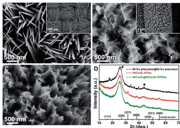
Fig. 2 (A–C) Typical SEM images: (A) Ni–Co precursor NWAs, (B) Ni–Co precursor@Ni–Co precursor NWSAs, and (C) NiCo<sub>2</sub>S<sub>4</sub>@NiCo<sub>2</sub>S<sub>4</sub> hybrid NTSAs. Inset shows the corresponding low-magnification SEM images. (D) XRD patterns of Ni–Co precursor@Ni–Co precursor NWSAs, NiCo<sub>2</sub>S<sub>4</sub> NTAs and NiCo<sub>2</sub>S<sub>4</sub>@NiCo<sub>2</sub>S<sub>4</sub> NTSAs. The peaks marked by “#” are arising from carbon cloth.
