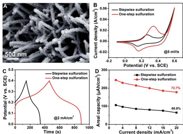
Fig. 7 (A) SEM image of  $\text{NiCo}_2\text{S}_4@/\text{NiCo}_2\text{S}_4$  hybrid NTSAs synthesized by the stepwise sulfuration method, (B–D) comparison of the electrochemical properties for the  $\text{NiCo}_2\text{S}_4@/\text{NiCo}_2\text{S}_4$  NTSAs obtained from different synthetic pathways: (B) CV curves, (C) GCD curves, and (D) rate capability.
