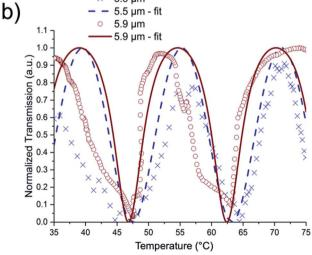
Fig. 4 (a) Transmission behaviour of a straight waveguide only without pronounced dips vs. a waveguide with a coupled micro-ring resonator. (b) Resonance behaviour during thermal tuning exemplarily shown at two selected wavelengths, corrected by the transmission behaviour of a straight waveguide at the respective wavelength to correct for nonring related transmission characteristics.
