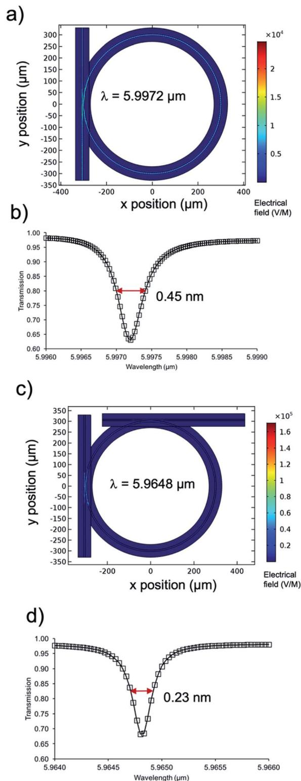
Fig. 1 (a) 2D FEM simulation of a 6  $\mu\text{m}$  GaAs micro-ring resonator showing the electrical field intensity. (b) Resonance dip for the plotted transmission of the throughput port of the structure shown in (a). (c) FEM simulated electrical field intensity for a micro-ring resonator with an out-coupling port. (d) Corresponding resonance dip at the throughput port of the structure shown in (c).
