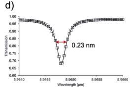
Fig. 1 (a) 2D FEM simulation of a 6  $\mu$ m GaAs micro-ring resonator showing the electrical field intensity. (b) Resonance dip for the plotted transmission of the throughput port of the structure shown in (a). (c) FEM simulated electrical field intensity for a micro-ring resonator with an out-coupling port. (d) Corresponding resonance dip at the throughput port of the structure shown in (c).
