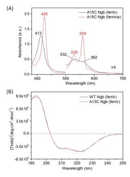
Fig. 2 Spectroscopic properties of A15C Ngb. (A) UV-Vis spectra in both oxidation states, and (B) CD spectrum in ferric state (10  $\mu M$  protein in 100 mM potassium phosphate buffer, pH 7.0, 25 °C), with WT Ngb shown for comparison.
