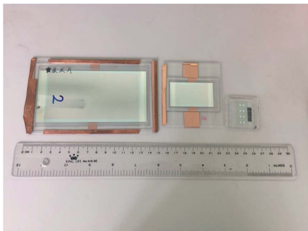
Fig. 16 A photograph of OLED devices of three different sizes in our laboratory, with substrate: 9 \times 15 \text{ cm}^2 , 7 \times 8 \text{ cm}^2 and 4 \times 4 \text{ cm}^2 .
