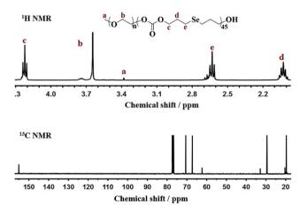
Fig. 1 NMR spectra of mPEG-b-CMP<sub>45</sub> in CDCl<sub>3</sub>.
