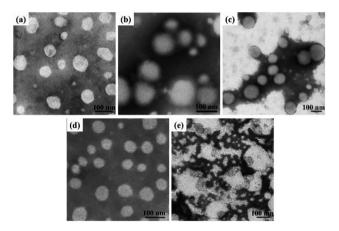
Fig. 3 TEM images of (a) copolymer mPEG-b-CMP $_{15}$  micelles (68 nm), (b) copolymer mPEG-b-CMP $_{30}$  micelles (101 nm), (c) copolymer mPEG-b-CMP $_{45}$  micelles (120 nm); and TEM images of mPEG-b-CMP $_{45}$  after reaction in (d) water and (e) 100  $\mu$ M H $_2$ O $_2$  aqueous solution after 24 h.
