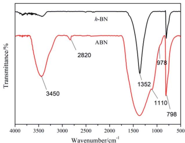
Fig. 5 FTIR spectra of h-BN and ABN.
