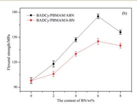
Fig. 8 Mechanical properties of BADCy/PBMAM/BN composites as a function of filler contents. (a) Unnotched impact strength; (b) flexural strength.
