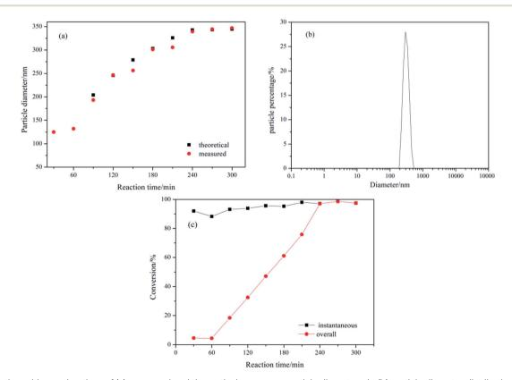
Fig. 3 Variation with reaction time of (a) measured and theoretical z-average particle diameter,  $d_z$ ; (b) particle diameter distribution of the final latex: (c) instantaneous and overall conversion.
