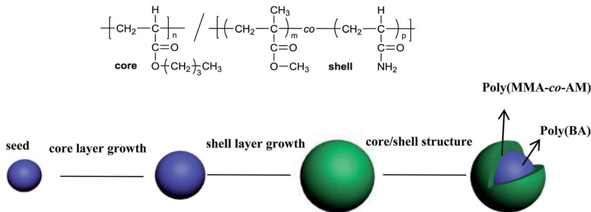
Fig. 1 Preparation procedure of PBAM.
