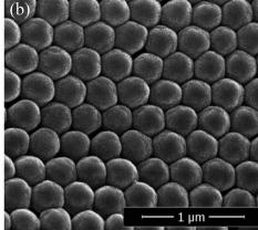
Fig. 4 PBMAM latex (a) TEM core-shell structure, (b) SEM particle distribution
