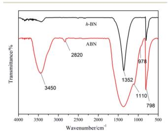
Fig. 5 FTIR spectra of h-BN and ABN.
