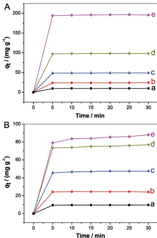
Fig. 8 Adsorbed capacity of  $\text{Fe}_3\text{O}_4/\text{MCM-41}$  as a function of contact time for (A) RhB and (B) MB at different initial concentrations of (a) 20, (b) 50, (c) 100, (d) 200 (e) 400  $\text{mg L}^{-1}$  at room temperature.
