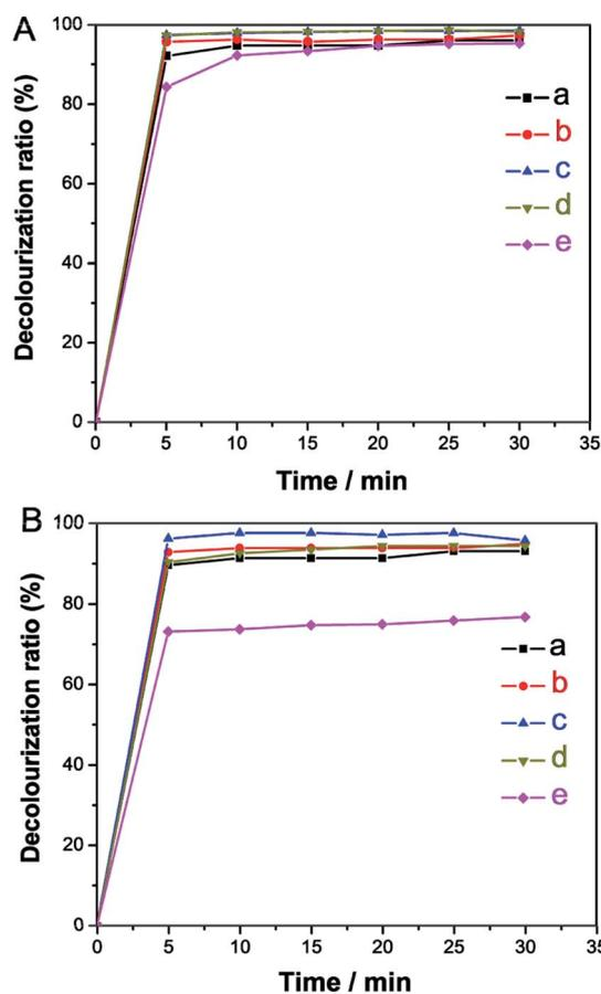
Fig. 7 Decolorization rates of (A) rhodamine B and (B) methylene blue solutions after adsorption using  $Fe_3O_4/MCM-41$  as adsorbent and magnetic separation at different time interval. The initial concentrations of solutions for rhodamine B: (a) 20, (b) 50, (c) 100, (d) 200 (e)  $400 \text{ mg L}^{-1}$ , and for methylene blue: (a) 10, (b) 20, (c) 50, (d) 100 (e)  $200 \text{ mg L}^{-1}$ .
