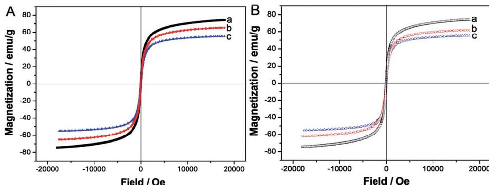
Fig. 2 (A) Magnetization curves of (a) bare  $\text{Fe}_3\text{O}_4$ , (b)  $\text{Fe}_3\text{O}_4/\text{C}_{10}\text{mimCl}$ , (c)  $\text{Fe}_3\text{O}_4/\text{C}_{10}\text{mimCl}/\text{C}_{16}\text{mimCl}$ , and (B) magnetization curves of (a) bare  $\text{Fe}_3\text{O}_4$ , (b)  $\text{Fe}_3\text{O}_4/\text{C}_{16}\text{mimCl}$ , (c)  $\text{Fe}_3\text{O}_4/\text{C}_{16}\text{mimCl}/\text{C}_{16}\text{mimCl}$ .
