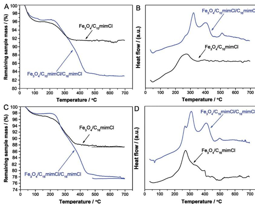
Fig. 3 (A) TGA and (B) DTA curves of  $\text{Fe}_3\text{O}_4/\text{C}_{10}\text{mimCl}$  and  $\text{Fe}_3\text{O}_4/\text{C}_{10}\text{mimCl}/\text{C}_{16}\text{mimCl}$ . (C) TGA and (D) DTA curves of  $\text{Fe}_3\text{O}_4/\text{C}_{16}\text{mimCl}$  and  $\text{Fe}_3\text{O}_4/\text{C}_{16}\text{mimCl}/\text{C}_{16}\text{mimCl}$ .
