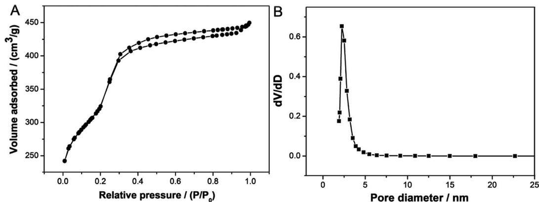
Fig. 6 (A)  $N_2$  adsorption–desorption isotherm of calcined sample prepared using  $C_{16}mimCl$  as template in the  $Fe_3O_4/C_{16}mimCl/C_{16}mimCl$  magnetic fluid, and (B) its BJH pore size distribution.
