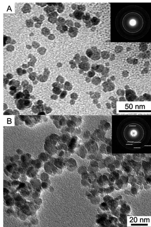
**Fig. 1** TEM images of (A) ionic liquid bilayer-stabilized  $\text{Fe}_3\text{O}_4/\text{C}_{10}\text{mimCl}/\text{C}_{16}\text{mimCl}$  and (B)  $\text{Fe}_3\text{O}_4/\text{C}_{16}\text{mimCl}/\text{C}_{16}\text{mimCl}$  particles. The insets show the corresponding electron diffraction images.
