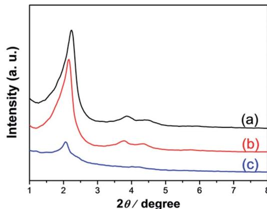
**Fig. 4** Small-angle XRD patterns of calcined samples prepared using  $C_{16}mimCl$  as template in the  $Fe_3O_4/C_{16}mimCl/C_{16}mimCl$  magnetic fluid with an initial molar ratio  $n(Fe_3O_4/C_{16}mimCl/C_{16}mimCl)/n(TEOS)$  of (a) 0.025, (b) 0.05 and (c) 0.10.
