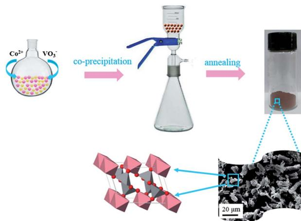
Fig. 1 Schematic of the synthesis of CoV<sub>2</sub>O<sub>6</sub>. Pink, gray and red represent Co, V, and O, respectively.
