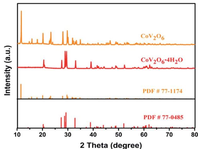
Fig. 2 XRD patterns of CoV<sub>2</sub>O<sub>6</sub>·4H<sub>2</sub>O and CoV<sub>2</sub>O<sub>6</sub>.
