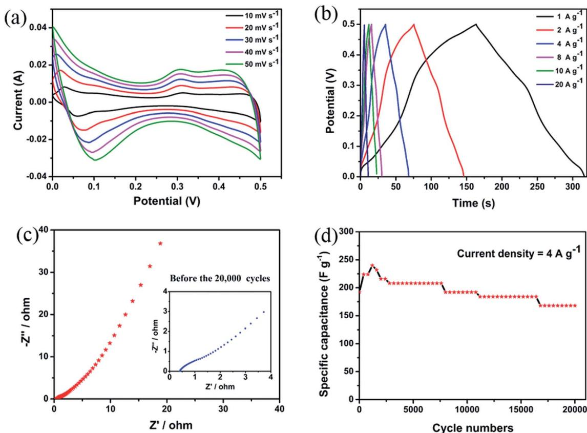
Fig. 4 (a) Cyclic voltammetry (CV) curves of  $\text{CoV}_2\text{O}_6$ . (b) Galvanostatic charge–discharge plots of  $\text{CoV}_2\text{O}_6$ . (c) EIS curves of  $\text{CoV}_2\text{O}_6$  (inset shows the magnified curve). (d) Cycle performance of  $\text{CoV}_2\text{O}_6$ .
