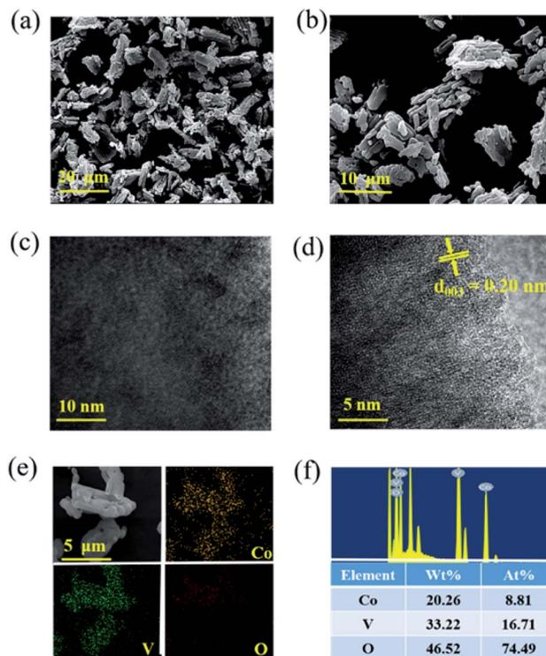
Fig. 3 (a and b) SEM images of  $\text{CoV}_2\text{O}_6$ , (c and d) TEM images of  $\text{CoV}_2\text{O}_6$ , (e) SEM image of  $\text{CoV}_2\text{O}_6$  and its corresponding elemental mapping images: Co, V, and O elements, and (f) the EDS spectrum of  $\text{CoV}_2\text{O}_6$ .
