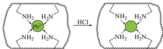
Fig. 12 Proposed reaction mechanism for Pb(II)-adsorption.
