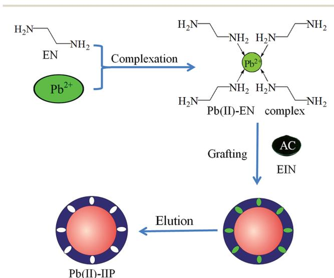
Fig. 1 Scheme for the preparation of Pb(II)-IIP.
