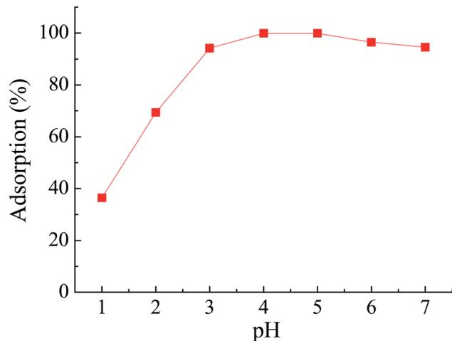
Fig. 6 Effect of pH on the adsorption of Pb(II) on Pb(II)-IIP.
