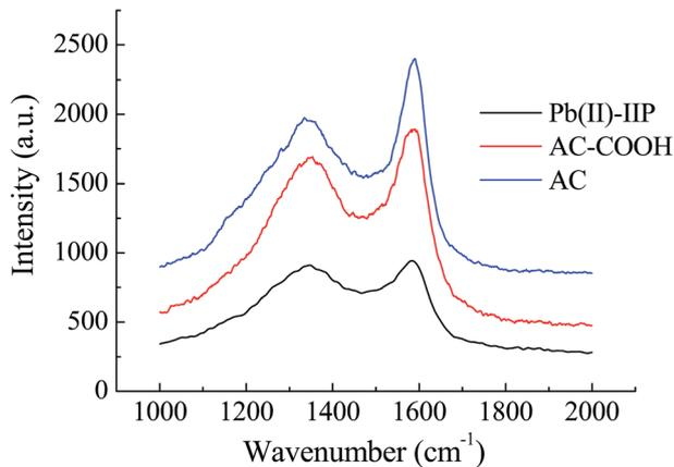
Fig. 3 Raman spectra of AC, AC-COOH and Pb(II)-IIP.
