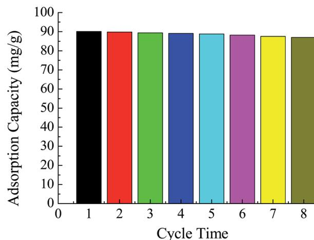
Fig. 11 Adsorption capacity of Pb(II)-IIP after eight cycles.
