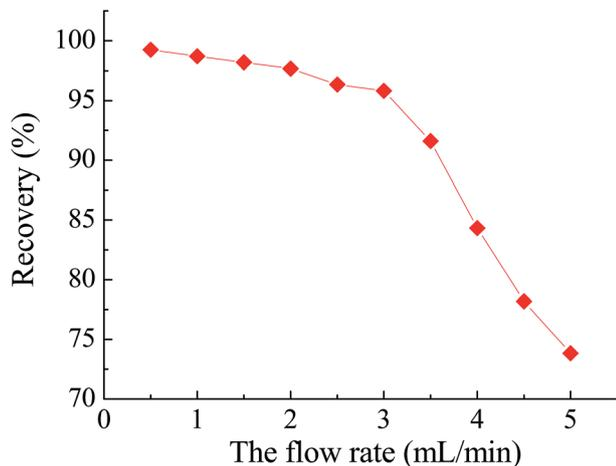
Fig. 8 Effect of solution flow rate on the recovery of Pb(II). Other conditions: volume 50 mL, pH 4.0, temperature 25 °C.
