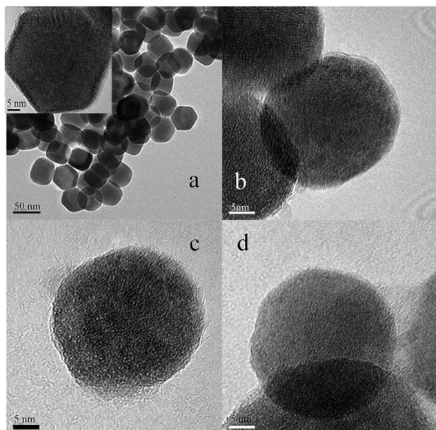
Fig. 1 TEM images of UCNP (a), UCNPs@SO<sub>3</sub>H (b), UCNPs@PO(OH)<sub>2</sub> (c) and UCNPs@GDN (d).
