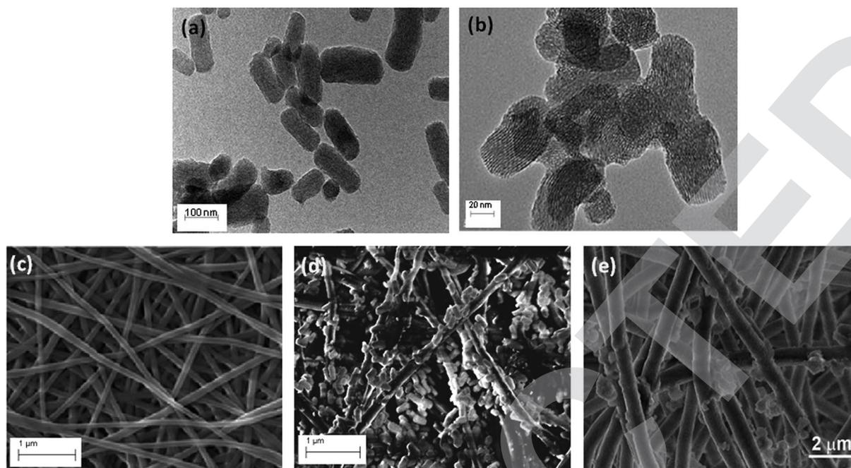
Fig. 2 HRTEM image for (a) MCM-NH<sub>2</sub>, and (b) MCM-PEI; and SEM images for (c) mPAN, (d) mPAN/MCM-NH<sub>2</sub> and (e) mPAN/MCM-PEI nanocomposites.
