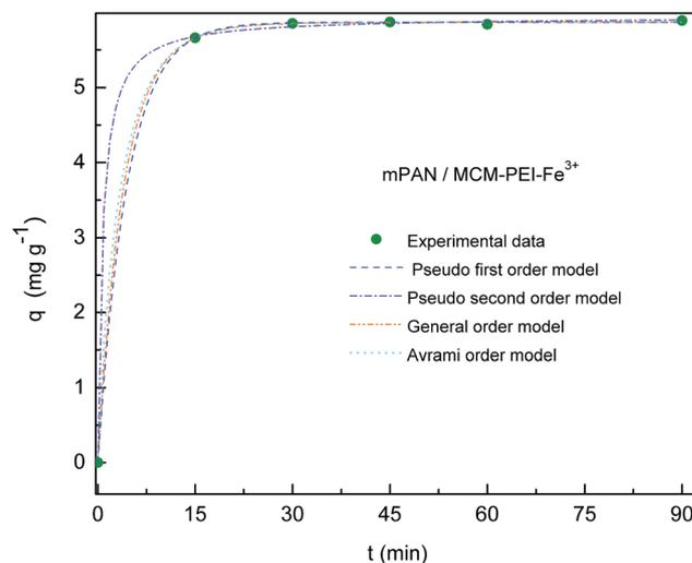
Fig. 7 Adsorption capacity for mPAN/MCM-PEI-Fe<sup>3+</sup>. Experimental data is represented by (●). Dashed and dot lines represents kinetic models used for fitting. Experimental conditions: initial concentration = 1 mg L<sup>-1</sup>, adsorbent amount = 20 mg, pH = 8.
