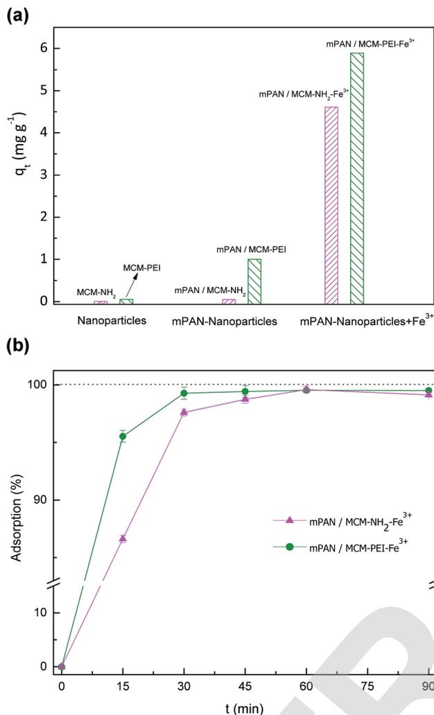
Fig. 5 (a) Adsorption percentage for comparison between nanoparticles, nanoparticles cross-linked to mPAN and with the incorporation of Fe<sup>3+</sup>; and (b) adsorption percentage for mPAN/MCM-NH<sub>2</sub>-Fe<sup>3+</sup> (—▲—) and mPAN/MCM-PEI-Fe<sup>3+</sup> (—●—) as a function of time.
