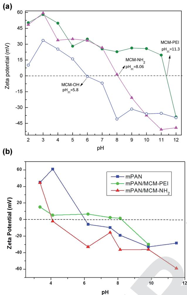
Fig. 3 Zeta potential and point-of-zero charge for (a) MCM-OH (—■—), MCM-NH<sub>2</sub> (—▲—) and MCM-PEI (—●—); (b) mPAN (—■—), mPAN/MCM-NH<sub>2</sub> (—▲—) and mPAN/MCM-PEI (—●—).
