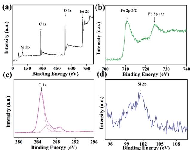
Fig. 3 XPS spectra of Acac-C@Fe<sub>3</sub>O<sub>4</sub>.
