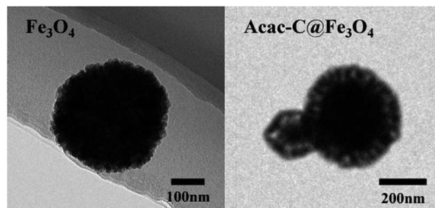
Fig. 5 SEM images of Fe<sub>3</sub>O<sub>4</sub> and Acac-C@Fe<sub>3</sub>O<sub>4</sub>.
