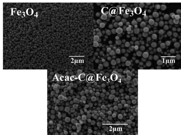
Fig. 4 SEM images of Fe<sub>3</sub>O<sub>4</sub>, C@Fe<sub>3</sub>O<sub>4</sub> and Acac-C@Fe<sub>3</sub>O<sub>4</sub>.
