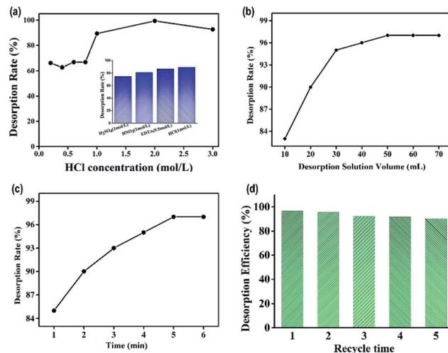
Fig. 8 (a) Influence of the concentration of  $\text{HCl}$  solution and the kind of desorption solution (inset) on the desorption efficiency; the influence of desorption solution volume (b) and desorption time (c) on the desorption efficiency; (d) desorption and regeneration of the as-prepared sorbent.
