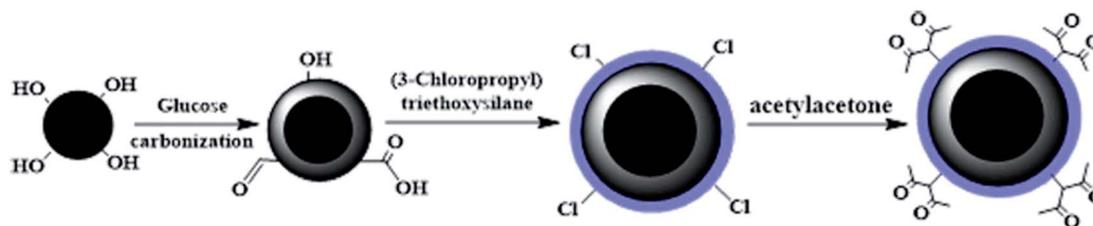
Scheme 1 Diagram of the Acac-C@Fe<sub>3</sub>O<sub>4</sub> magnetic material synthesis process.
