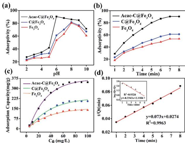
Fig. 6 Effect of pH (a), adsorption time (b), and initial concentration of  $\text{Pb}^{2+}$  (c) on the adsorption of  $\text{Pb}^{2+}$  onto Acac-C@ $\text{Fe}_3\text{O}_4$ , C@ $\text{Fe}_3\text{O}_4$  and  $\text{Fe}_3\text{O}_4$ ; (d) pseudo-second-order kinetic model for  $\text{Pb}^{2+}$  adsorption on Acac-C@ $\text{Fe}_3\text{O}_4$  sorbent (inset: pseudo-first-order kinetic model curve).
