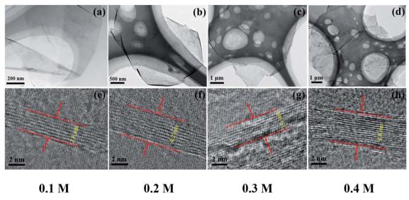
Fig. 3 (a-d) TEM images of graphene sheets of four conditions: 0.1 M, 0.2 M, 0.3 M, 0.4 M. (e-h) HRTEM images of four samples and the thickness of graphene sheets are 2.8, 4.2, 3.3, 4.8 nm, respectively.
