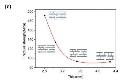
Fig. 5 (a) Schematic drawings of the uniaxial in-plane load-to-fracture of GP strips. (b) A schematic illustration of tension-shear transition, and how the interlayer crosslinks hinder the shear stress. (c) System diagram of graphene sheets thickness and fracture strength.
