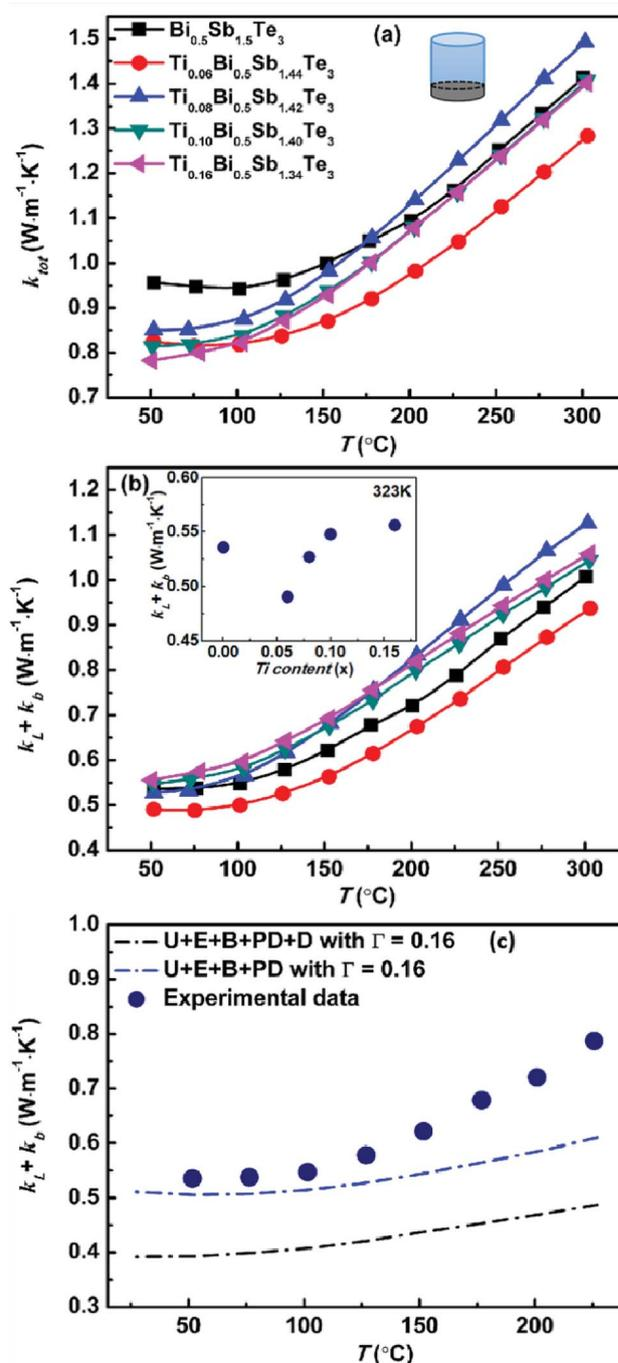
Fig. 3 (a) Temperature dependence of total thermal conductivity, (b) sum of the lattice and bipolar thermal conductivity for  $\text{Bi}_{0.5}\text{Ti}_x\text{Sb}_{1.5-x}\text{Te}_3$  samples and (c) measured  $\kappa_L + \kappa_b$  data points for  $\text{Bi}_{0.5}\text{Sb}_{1.5}\text{Te}_3$  pellet compared with calculated  $\kappa_L$  determined by different models.<sup>29</sup> The inset of (b) shows the  $\kappa_L + \kappa_b$  as a function of the Ti concentration at 323 K.
