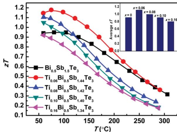
**Fig. 4**  $zT$  values of  $\text{Ti}_x\text{Bi}_{0.5}\text{Sb}_{1.5-x}\text{Te}_3$  samples.
