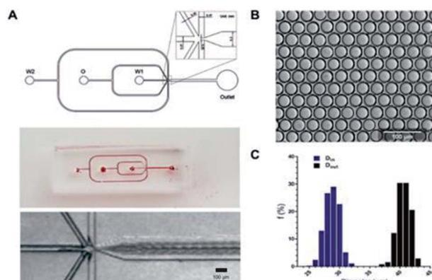
Fig. 2 Chip design and generation of W/O/W microdroplets. (A) Design and photographs of the one-step W/O/W microdroplet generator. Scale bar: 100  $\mu\text{m}$ . (B) Microphotograph of W/O/W microdroplets. Scale bar: 100  $\mu\text{m}$ . (C) The outer and inner diameters distribution of W/O/W microdroplets.
