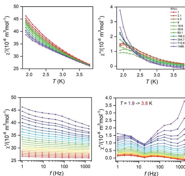
Fig. 3 Temperature and frequency dependent in-phase  $\chi'$  and out-of-phase  $\chi''$  molar susceptibilities for **1** at the applied external field  $B_{\text{DC}} = 0.1 \text{ T}$ . Lines serve as guide to the eye.
