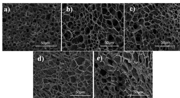
Fig. 6 SEM images of AEO-*n*-gels: (a) AEO<sub>3</sub>-gel, (b) AEO<sub>7</sub>-gel, (c) AEO<sub>9</sub>-gel, (d) AEO<sub>15</sub>-gel, (e) AEO<sub>23</sub>-gel.
