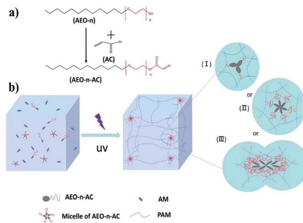
Fig. 2 (a) Schematic illustration for the synthesis and structure of AEO-*n*-AC and (b) the synthesis of (I) shorter-EO AEO<sub>3</sub>-gel, (II) long-EO AEO<sub>7</sub>-gel, or AEO<sub>9</sub>-gel (III) longer-EO AEO<sub>15</sub>-gel or AEO<sub>23</sub>-gel.
