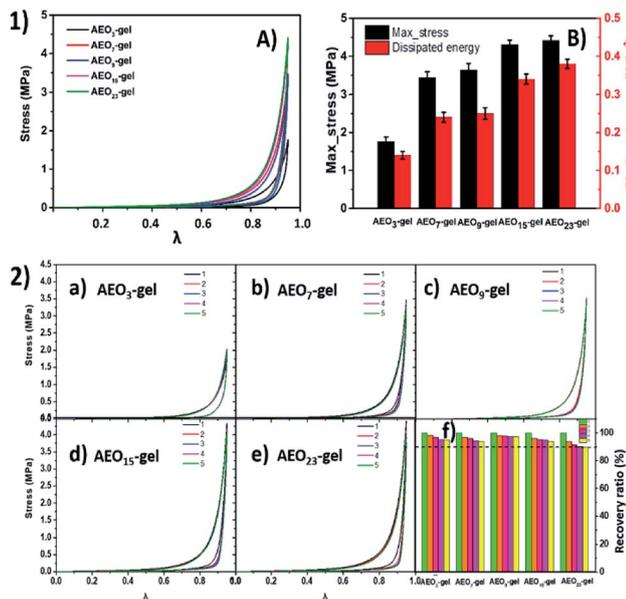
Fig. 9 (1-A) Compression loading-unloading curves at 0.95 compression ratio  $\lambda$  for AEO<sub>n</sub>-gels. (1-B) The corresponding stress and dissipated energy calculated from (A). (2-a–e) Cyclic compression loading-unloading curves for AEO<sub>n</sub>-gels. (2-f) the corresponding recovery ratio for (a–e).
