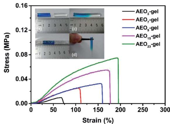
Fig. 10 Tensile stress–strain curves of the thermal healing AEO<sub>n</sub>-gels and the photographs of thermal healing process.
