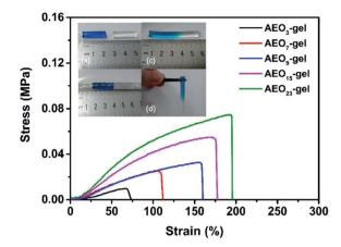
Fig. 10 Tensile stress-strain curves of the thermal healing  $AEO_n$ -gels and the photographs of thermal healing process.
