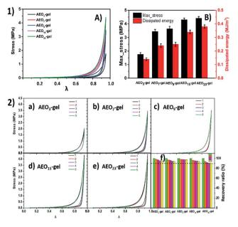
Fig. 9 (1-A) Compression loading-unloading curves at 0.95 compression ratio  $\lambda$  for AEO<sub>n</sub>-gels. (1-B) The corresponding stress and dissipated energy calculated form (A). (2-a-e) Cyclic compression loading-unloading curves for AEO<sub>n</sub>-gels. (2-f) the corresponding recovery ratio for (a-e).
