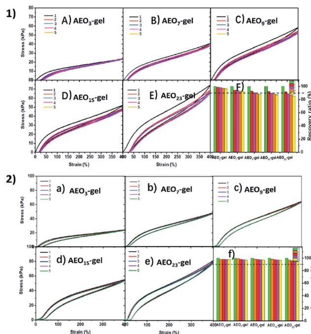
Fig. 8 Cyclic stress–strain curves of AEO-*n*-gels at the strain of 400% (1) without waiting time and (2) with 3 min waiting time. (F) and (f) the corresponding recovery ratio.
