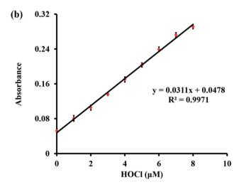
Fig. 3 (a) Absorption responses of probe TCFL (5  $\mu$ M) in the presence of different concentrations of HOCl (0–8  $\mu$ M) in PBS solution (5 mM, pH = 7.4). (b) The absorbance of TCFL at 490 nm as a function of HOCl concentration (0–8  $\mu$ M). Each spectrum was recorded 1 min after HOCl addition at 25 °C. Error bar = RSD (n=3).
