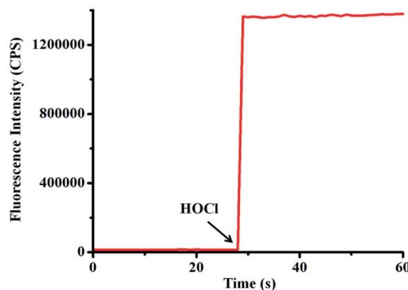
Fig. 1 Time-course of probe TCFL (5  $\mu\text{M}$ ) for monitoring HOCl (8  $\mu\text{M}$ ) in PBS solution (5 mM, pH = 7.4) at 25  $^\circ\text{C}$ .  $\lambda_{\text{ex}} = 470$  nm,  $\lambda_{\text{em}} = 515$  nm. Slit widths:  $W_{\text{ex}} = W_{\text{em}} = 1$  nm.
