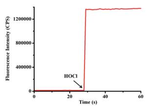
Fig. 1 Time-course of probe TCFL (5  $\mu$ M) for monitoring HOCl (8  $\mu$ M) in PBS solution (5 mM, pH = 7.4) at 25 °C.  $\lambda_{ex}$  = 470 nm,  $\lambda_{em}$  = 515 nm. Slit widths:  $W_{ex} = W_{em} = 1$  nm.
