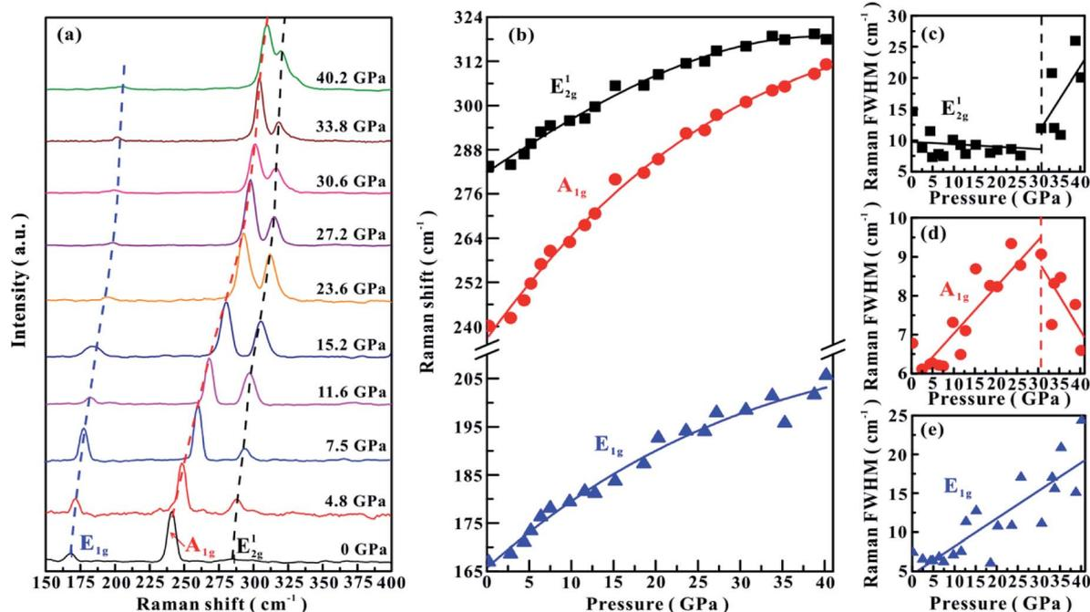
Fig. 2 (a) Raman spectroscopic results of MoSe<sub>2</sub> at representative pressure points under the hydrostatic condition. (b) The Raman shifts of three vibrational modes with increasing pressure. (c)–(e) The pressure dependence of FWHM for E<sub>2g</sub>, A<sub>1g</sub> and E<sub>1g</sub>, respectively. The dashed and solid lines serve as visual guides.
