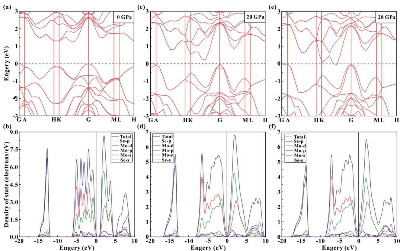
Fig. 8 (a), (c) and (e) The calculated band structure of MoSe<sub>2</sub> at representative pressures of  $\sim 0$ ,  $\sim 20$  and  $\sim 28$  GPa, respectively. (b), (d) and (f) The corresponding total density and projected density at  $\sim 0$ ,  $\sim 20$  and  $\sim 28$  GPa, respectively.
