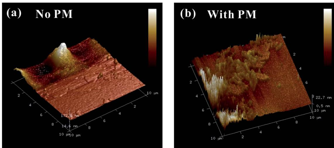
Fig. 7 (a) AFM images of decompressed MoSe<sub>2</sub> from  $\sim 37.5$  GPa under the non-hydrostatic condition. (b) AFM images of decompressed MoSe<sub>2</sub> from  $\sim 38.8$  GPa under the hydrostatic condition.
