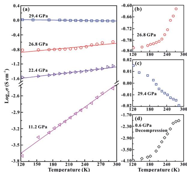
Fig. 5 (a) The temperature dependence of electrical conductivity for MoSe<sub>2</sub> at different pressure points under the hydrostatic condition. (b) The semiconducting state of MoSe<sub>2</sub> at  $\sim 26.8$  GPa. (c) The metallization of MoSe<sub>2</sub> at  $\sim 29.4$  GPa. (d) The semiconducting state of MoSe<sub>2</sub> after decompression.
