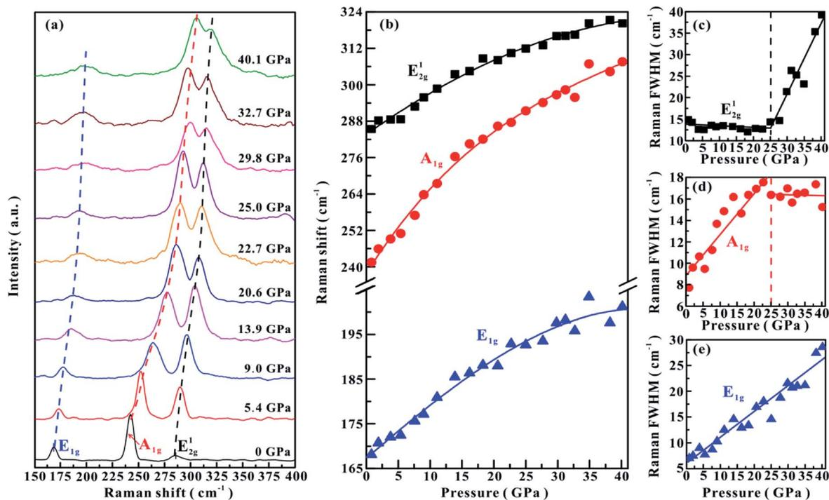
Fig. 1 (a) Raman spectra of MoSe<sub>2</sub> at representative pressure points under the non-hydrostatic condition. (b) The Raman shifts of three vibrational modes with increasing pressure. (c)–(e) The pressure dependence of FWHM for E<sub>2g</sub>, A<sub>1g</sub> and E<sub>1g</sub>, respectively. The dashed and solid lines serve as visual guides.
