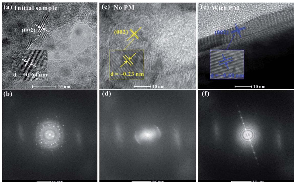
Fig. 6 (a), (c) and (e) The HRTEM image of the starting sample, the recovered MoSe<sub>2</sub> after decompression from  $\sim 40.0$  GPa under the non-hydrostatic condition, and the recovered MoSe<sub>2</sub> after decompression from  $\sim 39.6$  GPa under the hydrostatic condition, respectively. (b), (d) and (f) The corresponding fast Fourier transform (FFT) pattern. Scale bar, 10 nm.
