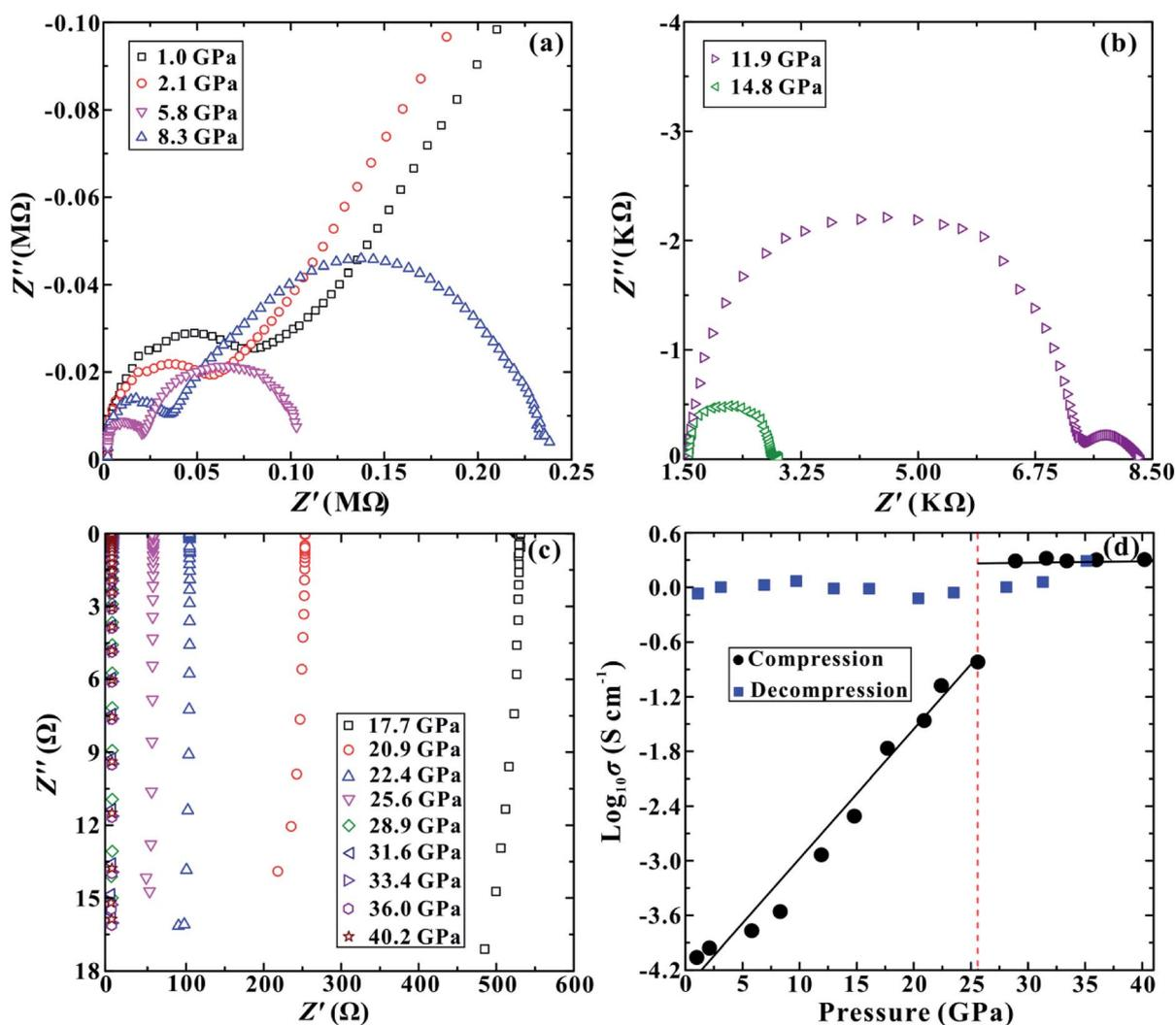
Fig. 3 (a)–(c) The impedance spectra of  $\text{MoSe}_2$  in pressure ranges of 1.0–40.2 GPa. The horizontal and vertical axes represent the real and imaginary parts of the complex impedance, respectively. (d) The pressure dependence of electrical conductivity for  $\text{MoSe}_2$  in the process of compression and decompression.
