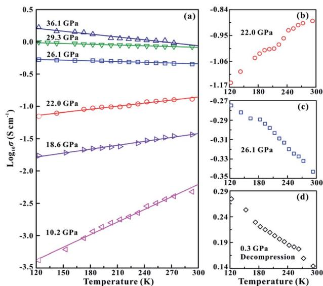
Fig. 4 (a) The temperature-dependent electrical conductivity of MoSe<sub>2</sub> at different pressure points under the non-hydrostatic condition. (b) The semiconducting state of MoSe<sub>2</sub> at  $\sim 22.0$  GPa. (c) The metallization of MoSe<sub>2</sub> at  $\sim 26.1$  GPa. (d) The metallic state of MoSe<sub>2</sub> after decompression.
