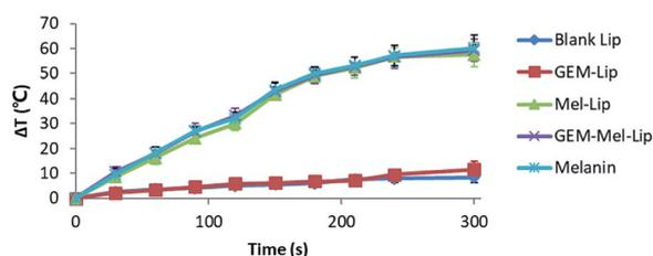
Fig. 5 Plot of temperature change of blank Lip, GEM-Lip (GEM concentration: 20 μg mL<sup>-1</sup>), Mel-Lip (melanin concentration: 180 μg mL<sup>-1</sup>), and GEM-Mel-Lip (GEM concentration: 20 μg mL<sup>-1</sup>, melanin concentration: 180 μg mL<sup>-1</sup>) under NIR irradiation (808 nm) for 5 min at a power density of 1.50 W cm<sup>-2</sup>.
