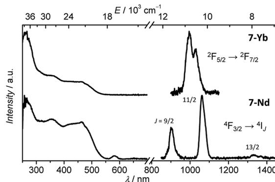
Fig. 3 (Left) Excitation upon monitoring either the  $\text{Yb}^{3+}$  emission signal at 980 nm or  $\text{Nd}^{3+}$  at 1064 nm, and (right) emission spectra upon excitation at 450 nm of 7-Nd and 7-Yb complexes at room temperature ( $\text{H}_2\text{O}$ ,  $1\text{ mg mL}^{-1}$ ).
