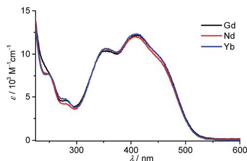
Fig. 1 Absorption spectra of **7-Ln** complexes (Ln = Nd, Gd, Yb) at room temperature ( $\text{H}_2\text{O}$ ,  $200 \mu\text{g mL}^{-1}$ ).
