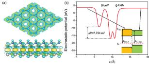
Fig. 7 (a) Isosurface with charge difference of 0.0004 e Å $^{-3}$ . (b) Potential drop across the interface of the g-GaN/BlueP vdW heterostructure. The yellow and cyan regions represent the gaining and losing, respectively, of electrons; the blue, gray, and cyan spheres represent P, Ga, and N atoms, respectively.
