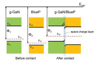
**Fig. 6** Energy-band diagrams of BlueP and g-GaN; schematic diagram of vdW heterostructure of BlueP and g-GaN.
