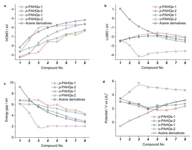
Fig. 3 Calculated energy levels and the redox potentials of p-PAHQs-1, p-PAHQs-2, o-PAHQs-1, o-PAHQs-2, and the referential acene derivatives. (a) HOMO energy level. (b) LUMO energy level. (c) Energy gap. (d) Redox potential.
