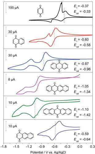
Fig. 4 Cyclic voltammetry profiles of p-PAHQs-1 and p-PAHQs-2 at a scan rate of 20 mV s<sup>-1</sup>. A cell with three-electrode configuration is used with glassy carbon, Pt wire, and AgCl/Ag electrodes serving as the working, counter, and reference electrodes, respectively. The composition of the electrolytes was 5 mM active materials and 1 M LiPF<sub>6</sub> in dimethylacetamide.
