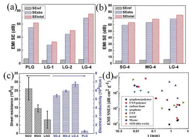
Fig. 5  $SE_{\text{ref}}$ ,  $SE_{\text{abs}}$  and  $SE_{\text{total}}$  at 10 GHz of (a) the PLG, LG-1, LG-2, LG-4 films, (b) the SG-4, MG-4, LG-4 films; (c) electrical conductivity of GO films and graphene films; (d) EMI SSE/ $t$  versus thickness of the graphene films, in comparison to different materials in the previous literature, and  $t$  represents thickness.
