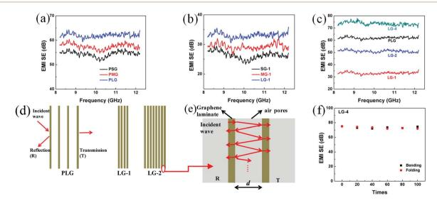
Fig. 4 The EMI SEs of (a) the PG films, (b) the graphene films compressed with one PG film, (c) the graphene films made of large-sized flakes; (d) an ideal multi-layer model for PLG and compressed graphene films composed of graphene laminates and insulated air pores; (e) schematic representation of a local multi-layer model composed of two graphene laminates and insulated pores between two graphene laminates; (f) EMI SEs of the LG-4 film after bending and folding.
