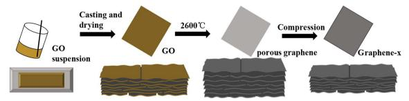
Schematic illustration of preparation process of graphene films (x represents the number of PrGO films were compressed together).
