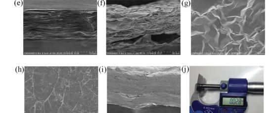
Fig. 2 Morphology and structural characterization of GO and graphene films. (a) Corresponding histograms of GO flakes size distribution; SEM images of: (b) small-size flakes, (c) medium-size flakes and (d) large-size flakes; cross-section SEM images of (e) LGO film; (f) PLG film; top views of (g) PLG film, (h) LG-1 film; cross-section SEM images of (i) LG-8 film; (j) picture of thickness measurement.
