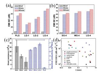
Fig. 5  $\,$  SE<sub>ref</sub>, SE<sub>abs</sub> and SE<sub>total</sub> at 10 GHz of (a) the PLG, LG-1, LG-2, LG-4 films, (b) the SG-4, MG-4, LG-4 films; (c) electrical conductivity of GO films and graphene films; (d) EMI SSE/t versus thickness of the graphene films, in comparison to different materials in the previous literature, and t represents thickness.
