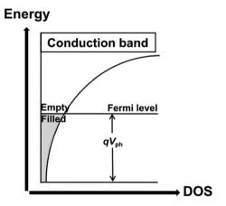
Fig. 3 Illustration of the dependence of the trapped electron density on the photovoltage for an exponential distribution of traps.<sup>17</sup>
