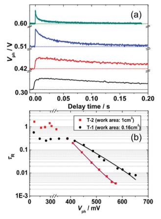
Fig. 5 (a) Representative kinetic traces of transient photovoltage (TPV) at specific  $V_{\rm ph}$ . (b) Semi-logarithmic plots of the TPV-determined  $\tau_{\rm R}$  as a function of  $V_{\rm ph}$  for T-1 and T-2. Solid lines were derived by fitting the data from  $V_{\rm ph}$  > 400 mV to an exponential model function [eqn (5)].
