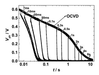
Fig. 2 Representative kinetic traces of the overall photovoltage  $(V_{ph})$  for a DSSC device under open circuit conditions, and the charge extraction kinetics at the indicated times recorded by switching the DSSC to a short circuit condition.
