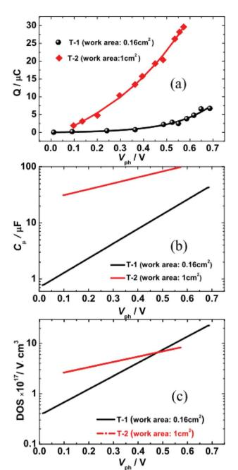
Fig. 4 (a) Extracted charge as a function of photovoltage  $(V_{ph})$ . (b and c) Semi-logarithmic plots of chemical capacitance  $C_{\mu}$  (b) and DOS (c) against  $V_{ph}$  for T-1 and T-2 solar cells.
