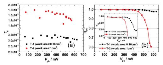
Fig. 6 (a) The TPC-determined electron collection time constant  $\tau_{\rm C}$  as a function of  $V_{\rm ph}$  for T-1 and T-2. (b) eqn (6)-determined electronic collection efficiency  $\eta_{cc}$  as a function of  $V_{ph}$  for T-1 and T-2. Inset: to show the  $\eta_{cc}$  of T-1 in detail, the region from 0.97 to 1 on the y-axis has been enlarged.
