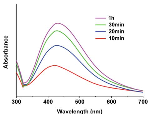
Fig. 2 UV-Vis absorption spectra of PEO/AgBF<sub>4</sub>/HMIM<sup>+</sup>BF<sub>4</sub><sup>-</sup> solution with heating time.
