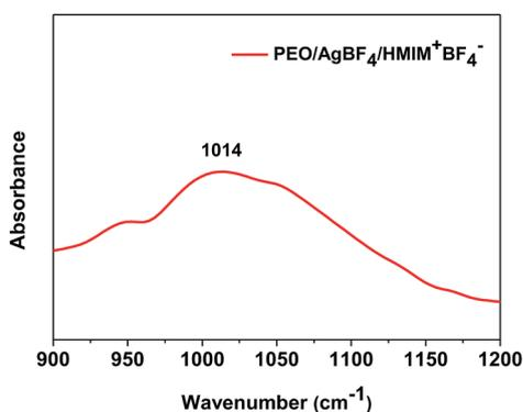
Fig. 3 FT-IR spectra of PEO/AgBF<sub>4</sub>/HMIM<sup>+</sup>BF<sub>4</sub><sup>-</sup> complex.
