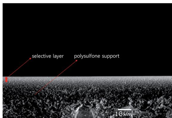
Fig. 1 Cross-sectional SEM image of PEO/AgBF<sub>4</sub>/HMIM<sup>+</sup>BF<sub>4</sub><sup>-</sup> composite membrane.
