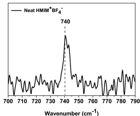
Fig. 6 Raman spectrum of neat HMIM<sup>+</sup>BF<sub>4</sub><sup>-</sup>.
