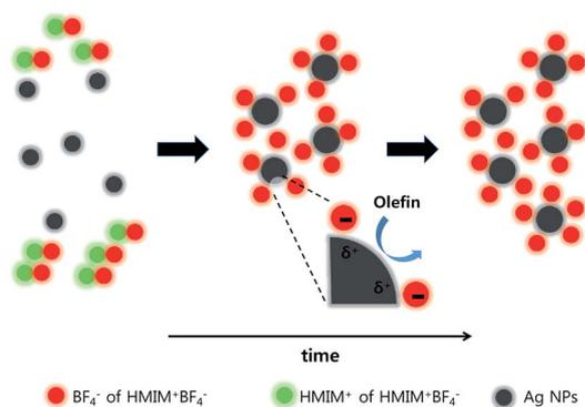
Scheme 1 Ag NPs formation in PEO/AgBF<sub>4</sub>/HMIM<sup>+</sup>BF<sub>4</sub><sup>-</sup> composite membrane upon heating.
