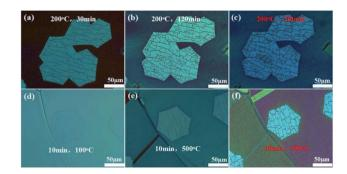
Fig. 2 Optical microscopy images of graphene domains after etching. (a-c) Degree of etching depending on the etching times of 30, 120, and 240 min, respectively. The etching temperature was 200 °C. (d-f) Degree of etching depending on the etching temperatures of 100, 500, and 950 °C. The etching time was 10 min. The gas flow rate of etching was 2:5 (200 sccm H<sub>2</sub> and 500 sccm Ar).
