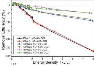
Fig. 16 Effects of CO $_2$  on the NTP denitration performance, (a) effects of CO $_2$  on DBD outlet gas concentration in the system of 1500  $\mu$ L L $^{-1}$  NO + 14% O $_2$  + 5.1% H $_2$ O + 76.2% N $_2$ . (b) Effects of CO $_2$  on the NTP removal efficiency at different initial NO concentration in 14% O $_2$  + 5.1% H $_2$ O + 76.2% N $_2$  + NO.
