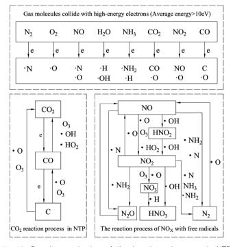
Fig. 18 Reaction mechanism of diesel engine exhaust gas in NTP system.
