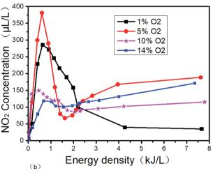
Fig. 9 Effect of NTP at different energy density in  $O_2/N_2$  system. (a) NO varies with energy density, (b)  $NO_2$  varies with energy density.
