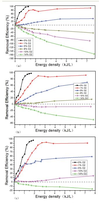
Fig. 11 Denitration performance of NTP in NO/O<sub>2</sub>/N<sub>2</sub> system, (a) 500  $\mu L L^{-1} NO + O_2$ , (b) 1000  $\mu L L^{-1} NO + O_2$ , (c) 1500  $\mu L L^{-1} NO + O_2$
