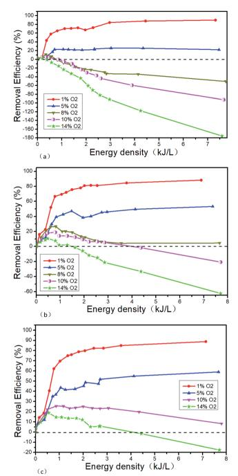
Fig. 12 Denitration performance of NTP in NO/NH<sub>3</sub>/O<sub>2</sub>/N<sub>2</sub> system, (a)  $500 \mu L L^{-1} NO + 500 \mu L L^{-1} NH_3 + O_2$ , (b) 1000 μL  $L^{-1} NO + 1000 \mu L$  $L^{-1} NH_3 + O_2$ , (c) 1500  $\mu L L^{-1} NO + 1500 \mu L L^{-1} NH_3 + O_2$ .
