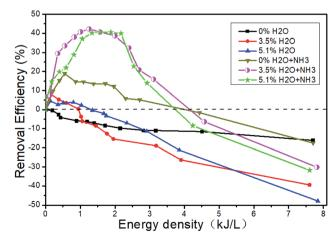
Fig. 14 Effect of H<sub>2</sub>O and NH<sub>3</sub> on the removal efficiency.
