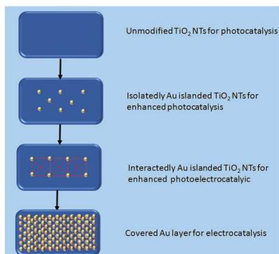
Scheme 1 Isolated/interacting Au islands on TiO<sub>2</sub> NTs for photocatalytic/photoelectrocatalytic switching.
