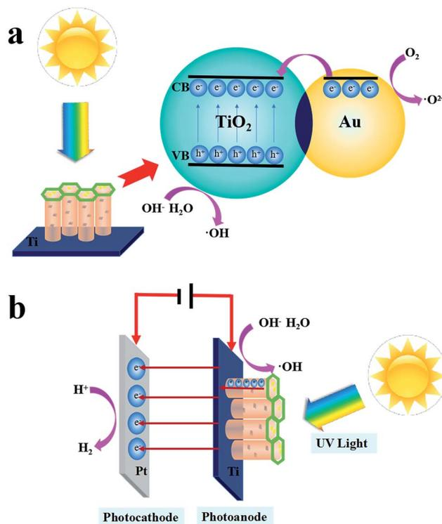
Scheme 2 (a) PC mechanism of the Au/TiO<sub>2</sub> NTs; (b) PEC mechanism of the Au/TiO<sub>2</sub> NTs.
