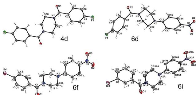
Fig. 9 Molecular structures of **4d**, **6d**, **6f**, and **6i** with atom labeling scheme (ORTEP plots, thermal displacement ellipsoids are shown with 50% probability at  $-150\text{ }^{\circ}\text{C}$ ).
