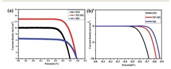
Fig. 6 J-V characteristics of DSSCs (a) under illumination with light intensity of 100 mW cm<sup>-2</sup> and (b) in the dark condition.
