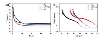
Fig. 8 (a) The open-circuit voltage decay profiles and (b) the electron lifetime- $V_{\rm OC}$  curves of DSSCs.
