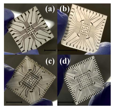
Fig. 4 Optical micrographs of the bottom view of (a)  $5 \times 5$  and (b)  $6 \times 6$  ink casted device. Top view or  $8 \times 8$  ink casted device showing (c) 16 electrodes on the top side and (d) 48 electrodes on the bottom side. Scale bar in figures correspond to 10 mm.
