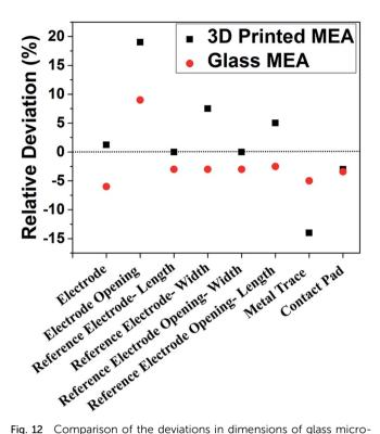
Fig. 12 Comparison of the deviations in dimensions of glass micromachined and 3D printed MEAs (values represent a measured average of N=3 devices for both MEA types). The values show the relative deviation from the measured average to the designed dimension.
