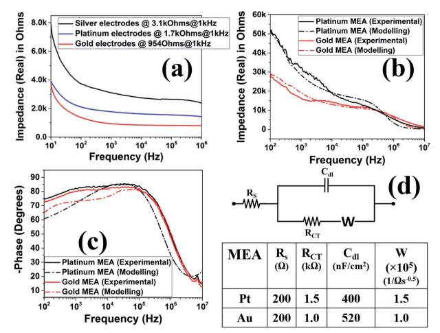
Fig. 11 Full spectrum impedance graphs for (a) 450  $\mu$ m diameter electrodes and (b) 50  $\mu$ m  $\times$  50  $\mu$ m laser micromachined electrodes (as obtained experimentally and by modelling), (c) phase (degrees) of the 50  $\mu$ m  $\times$  50  $\mu$ m laser micromachined electrodes (as obtained experimentally and by modelling). (d) Randles equivalent model used for extraction of the MEA circuit elements and the estimated values for the nano-porous platinum and nano-gold MEAs.
