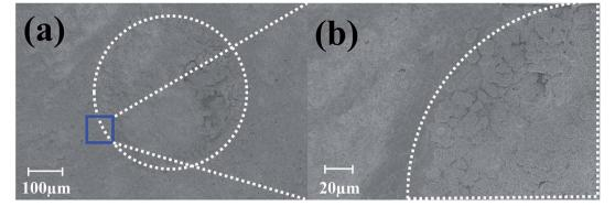
Fig. 7 (a) SEM images depicting pulsed electroplated platinum atop the silver ink casted electrodes with (b) depicting filling of the electrode edges.
