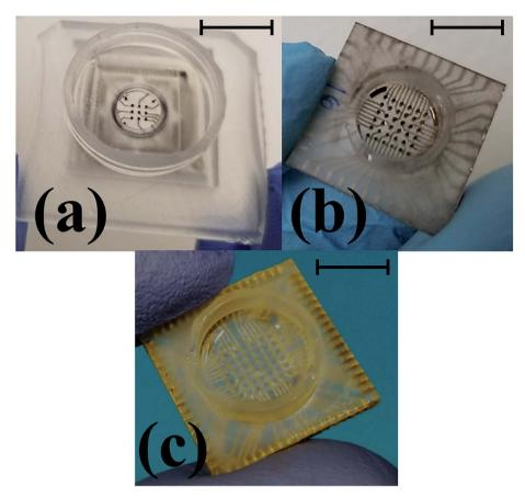
Fig. 10 Optical images of the final fabricated device ready for testing transitioning from the previously reported  $3 \times 3$  array<sup>22</sup> (a) to a monolithically integrated  $6 \times 6$  array (b) and a high density  $8 \times 8$  array MEA (c). Scale bar in the images corresponds to 10 mm.
