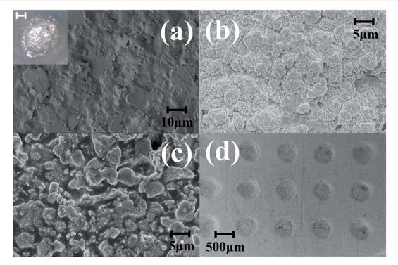
Fig. 8 SEM images of (a) silver electrodes with photo micrograph of ink casted silver electrode as inset (scale bar of the inset image corresponding to  $100 \mu m$ ), (b) nano-porous platinum electrode, and (c) nano-gold electrodes. (d) SU-8 CPSC MEA device after platinum electroplating showing a conformal layer of uniform insulation.
