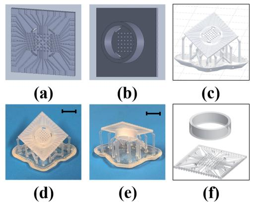
Fig. 2 Stages of MEA fabrication: (a and b) SolidWorks model (bottom and top views of  $6 \times 6$  design), (c) Preform model, (d and e) printed device (bottom and top views) and (f)  $8 \times 8$  design in which the MEA chip and culture well are printed as two separate parts and affixed together with a biocompatible epoxy. Scale bars in (d) and (e) correspond to 10 mm.
