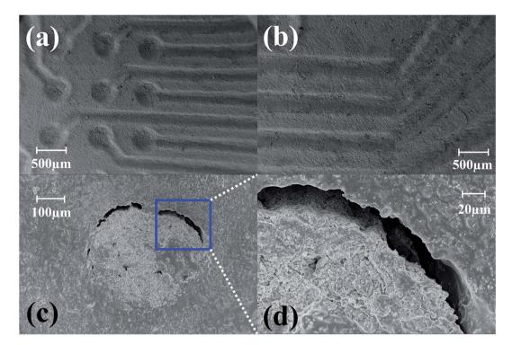
Fig. 5 (a) SEM imaging depicting the microelectrodes transitioning smoothly to the traces as seen from the bottom side of the MEA chip. (b) Adjacent traces separated by a gap of  $\sim$ 80  $\mu$ m. SEM image of ink casted electrodes with (c) unfilled electrode edges and (d) close up of (c).
