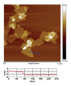
Fig. 2 AFM topography and cross section of GO.
