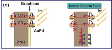
Fig. 7 Illustration of the PEC mechanism of (a) ZNR/AuPd. (b) ZNR@Gr. and (c) ZNR@Gr/AuPd.
