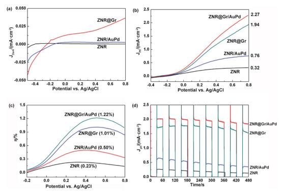
Fig. 5 (a) Dark current density of ZNR, ZNR/AuPd, and ZNR@Gr. (b) Photo current density and (c) photoconversion efficiency of ZNR, ZNR/AuPd, ZNR@Gr, and ZNR@Gr/AuPd under AM 1.5 G illumination (100 mW cm<sup>-2</sup>). (d) Intermittent photocurrent density-time curves with 60 s for a period.
