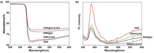
(a) UV-visible spectra of ZNR, ZNR@Gr, ZNR/AuPd, and ZNR@Gr/AuPd; (b) PL spectra of ZNR, ZNR@Gr, ZNR/AuPd, and ZNR@Gr/AuPd.
