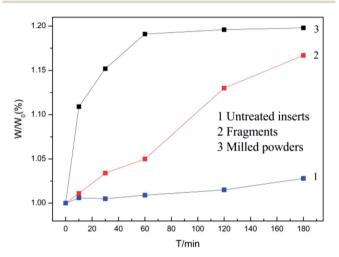
Fig. 3 Weight ratios versus oxidation time.
