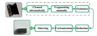
Fig. 2 Recycling waste inserts by the oxidation and reduction-carbon process
