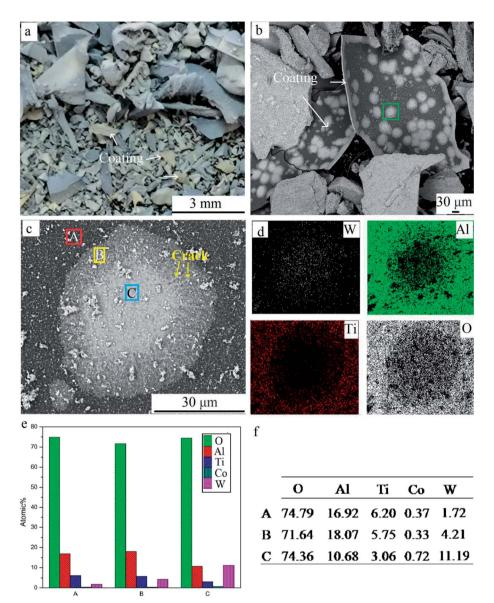
Fig. 8 Coatings delaminated from the whole inserts. (a) Macrographs; (b) SEM image; (c) high magnification SEM image; and (d-f) EDS results of three points.
