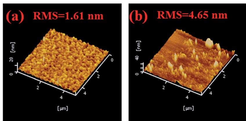
Fig. 6 The AFM of C-HTLs film with doping structure. (a) MoO<sub>3</sub> (3 nm)/CBP:16% MoO<sub>3</sub> (consist with E-3). (b) MoO<sub>3</sub> (3 nm)/CBP:50% MoO<sub>3</sub> (higher doping ratio).
