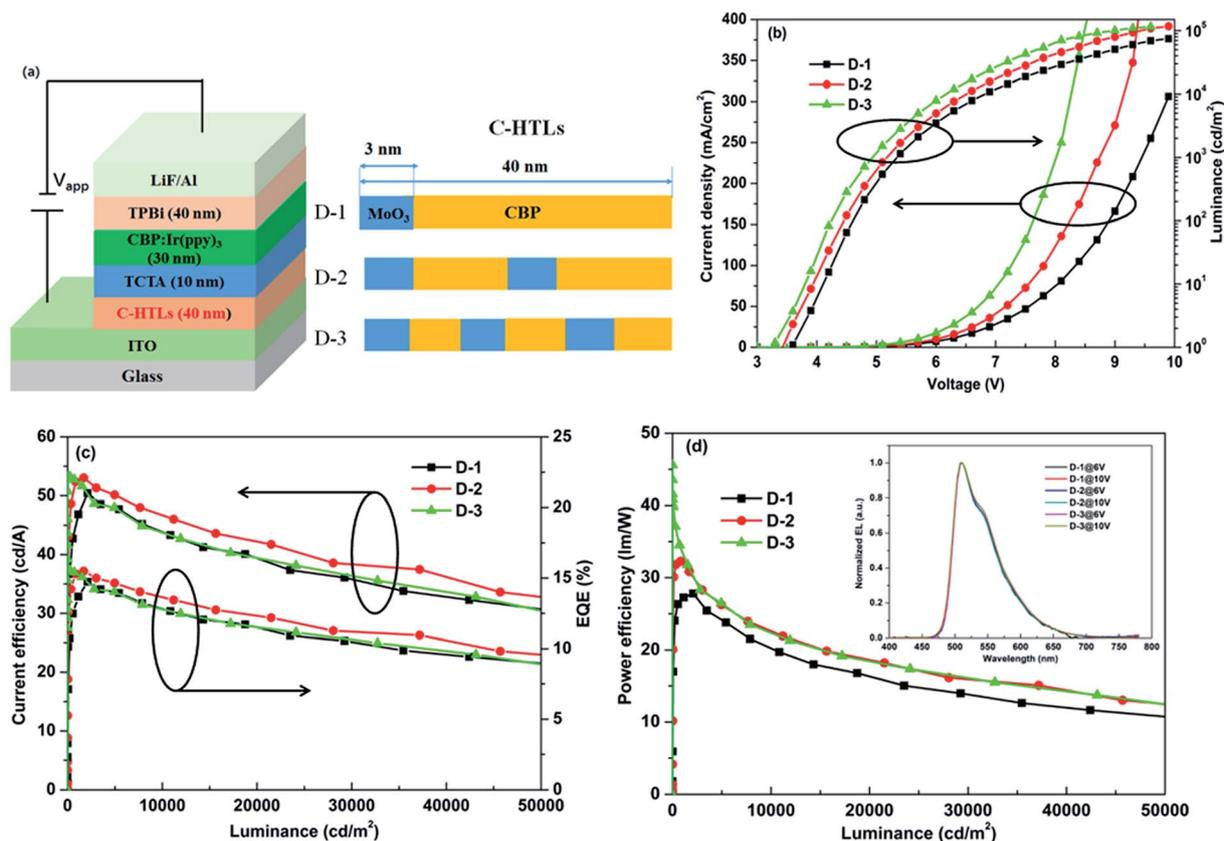
Fig. 1 Device structure and EL performances. (a) Device structure. (b) Current density–voltage–luminance curves. (c) Current efficiency–luminance–EQE curves. (d) Power efficiency–luminance curves. Inset is the EL spectra under different voltages.
