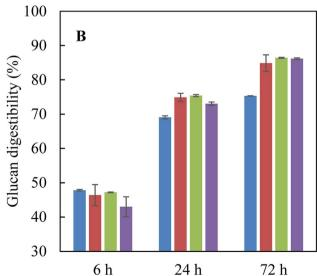
Fig. 1 Effect of glycerol-rich pretreatment hydrolysate (0%, 2%, 5% and 7.5% glycerol) on enzymatic hydrolysis. (A) In citric buffer; (B) with pretreatment hydrolysate.
