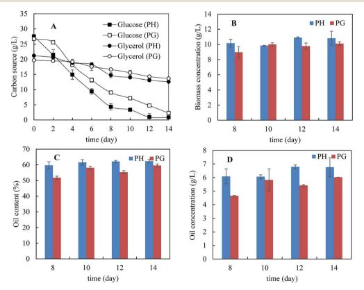
Fig. 2 Fermentation profile of the M. isabellina strain grown on pretreated bagasse enzyme hydrolysate with pretreatment hydrolysate and pure glycerol, respectively. (A) Kinetics of carbon source consumption; (B) fungal biomass concentrations; (C) oil contents; (D) oil concentrations. PH: pretreatment hydrolysate; PG: pure glycerol.
