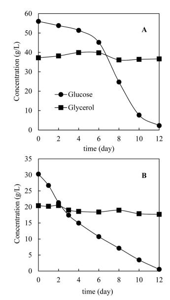
Fig. 3 Kinetics of carbon source consumption in a 1 L bioreactor. (A) Initial carbon sources: 56.0 g  $\rm L^{-1}$  glucose + 37.2 g  $\rm L^{-1}$  glycerol; (B) 30.2 g  $\rm L^{-1}$  glucose and 20.4 g  $\rm L^{-1}$  glycerol.
