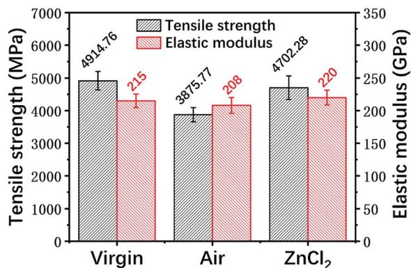
Fig. 12 Single fiber tensile strengths and elastic moduli of the different fiber samples.
