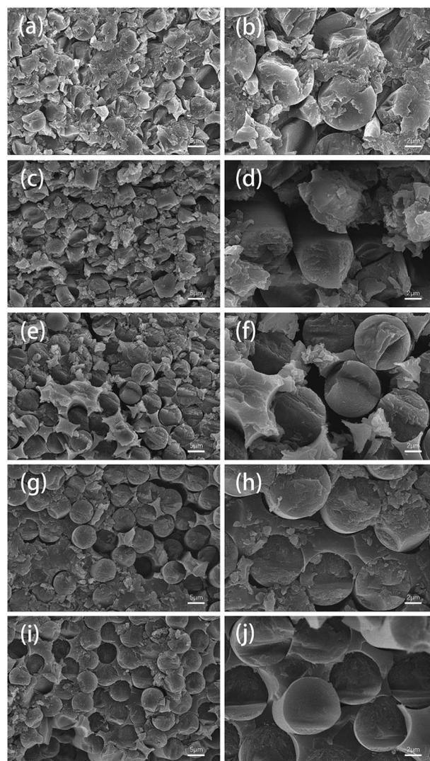
Fig. 14 SEM images of the fracture surfaces of composites made from (a and b) virgin fibers, (c and d) air-reclaimed fibers, (e and f) ZnCl<sub>2</sub>-reclaimed fibers, (g and h) air-reclaimed fibers after sizing, and (i and j) ZnCl<sub>2</sub>-reclaimed fibers after sizing.
