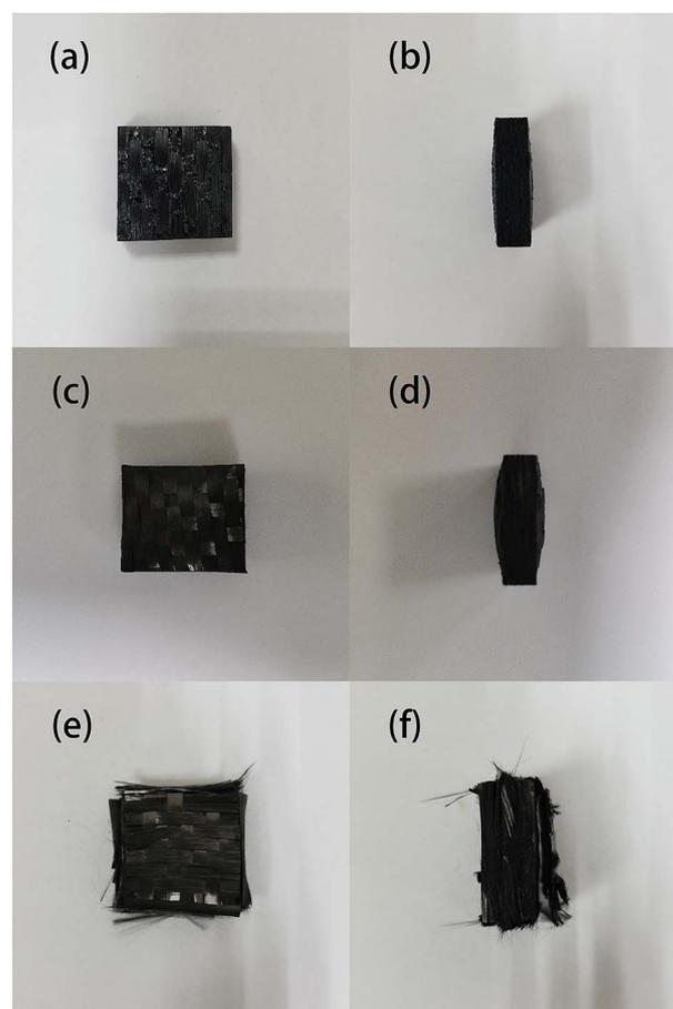
Fig. 4 The appearance of samples degraded in air at 360 °C for 40 min: (a) front view, (b) side view; in air at 450 °C for 40 min: (c) front view, (d) side view; and samples degraded with ZnCl<sub>2</sub> at 360 °C for 40 min: (e) front view, (f) side view.
