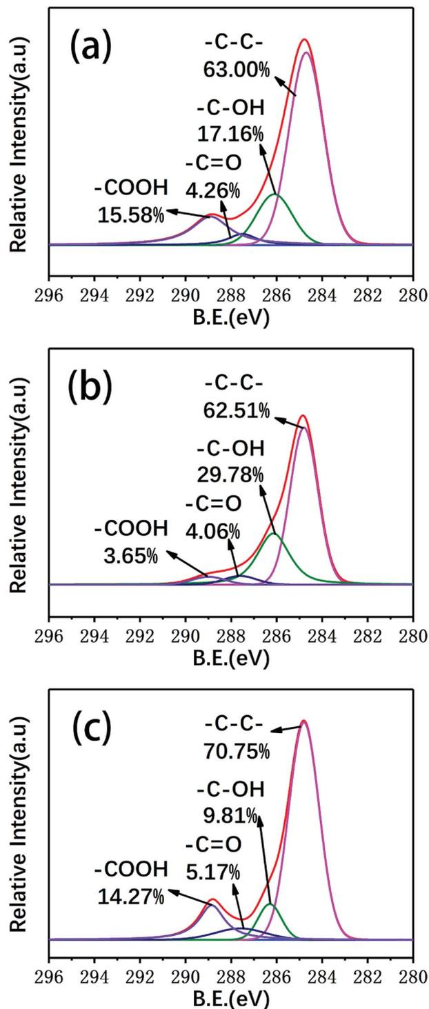
Fig. 9 The general XPS spectra and deconvolution of the C 1s XPS spectra of (a) the virgin fibers and the fibers reclaimed (b) in air and (c) with ZnCl<sub>2</sub>.
