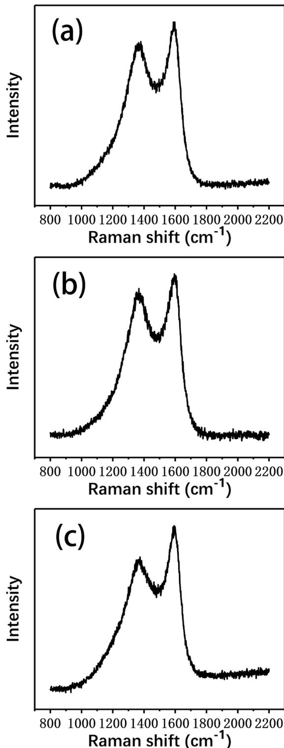
Fig. 10 The Raman spectra of (a) the virgin fibers and the fibers reclaimed (b) in air and (c) with ZnCl<sub>2</sub>.
