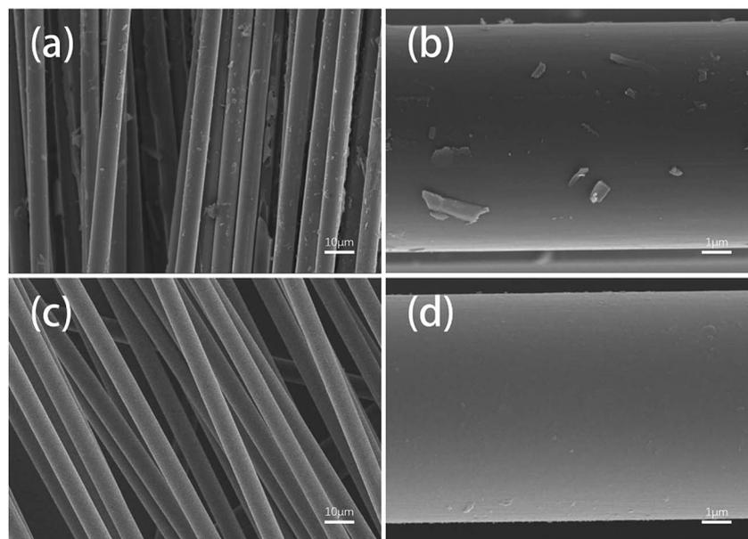
Fig. 7 SEM images of the fiber samples reclaimed (a and b) in air and (c and d) with  $\text{ZnCl}_2$ .
