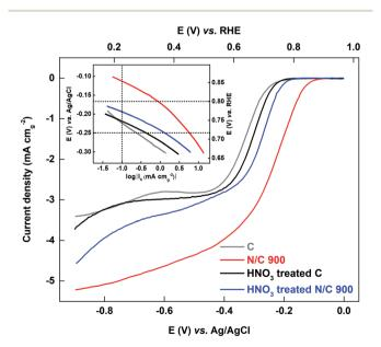
Fig. 8 ORR voltammograms of C and N/C 900 with their respective HNO $_3$  treated catalysts recorded in oxygen-saturated 0.1 M KOH solution (pH 13) at a scan rate of 20 mV s $^{-1}$  at 1600 rpm. Inset shows the Tafel plot of the respective catalysts.
