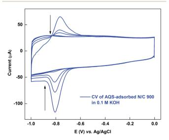
Fig. 4 Voltammogram of AQS-adsorbed N/C 900 potential cycled in argon-saturated 0.1 M KOH (pH 13) at 20 mV s<sup>-1</sup> scan rate.
