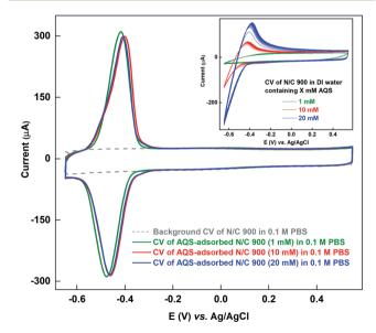
Fig. 3 Voltammogram of AQS-adsorbed N/C 900 recorded in argon-saturated AQS-free 0.1 M PBS (pH 7) at 20 mV s $^{-1}$  scan rate after cycling in AQS-containing DI water. Gray dotted line represents the background voltammogram of N/C 900 recorded in AQS-free argon-saturated 0.1 M PBS (pH 7). Inset shows the voltammograms of N/C 900 for the potential cycling in aqueous AQS solutions of different concentrations.
