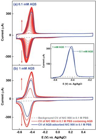
Fig. 2 Voltammograms of N/C 900 recorded in argon-saturated 0.1 M PBS (pH 7) at 20 mV s $^{-1}$  scan rate at different conditions. Background CV (gray); cycling CV in 0.1 mM (a), and 1 mM (b) AQS (red); and CV of AQS-adsorbed electrode after potential cycling in 0.1 mM (a) and 1 mM (b) AQS (blue). Inset shows the overlapping voltammograms (oxidation peak from the forward cycle) of the AQS-adsorbed electrode after potential cycling in 0.1 mM and 1 mM AQS.
