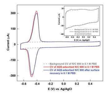
Fig. 5 Voltammograms of N/C 900 catalyst recorded in argon-saturated 0.1 M PBS (pH 7) at 20 mV s<sup>-1</sup> scan rate at different conditions; background (gray), AQS-adsorbed electrode (red), and with the recovered surface (blue). The inset represents the comparison of the background voltammograms of the initial and the recovered surfaces of N/C 900 after electrochemical cleaning in KOH media.
