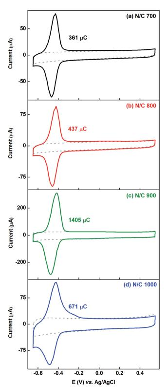
Fig. 6 Voltammograms of the AQS-adsorbed N/C 700 (a), N/C 800 (b), N/C 900 (c), and N/C 1000 (d) in argon-saturated 0.1 M PBS (pH 7) at 20 mV s $^{-1}$  scan rate. The dotted gray line represents the background voltammogram of the respective catalyst.
