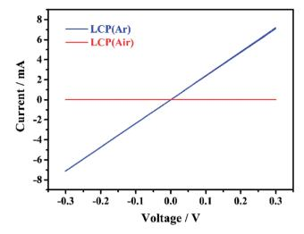
Fig. 7 Current-voltage plots (3 cycles each) for LiCoPO<sub>4</sub> samples fired in Ar and air, respectively, cycling at scanning rate of 20 mV s<sup>-1</sup>. showing the ohmic behaviour of the samples (labels explained in Scheme 1)
