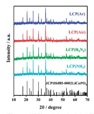
Fig. 2 XRD patterns of LiCoPO $_4$  samples heated under Ar, air,  $5\%~H_2/N_2$  and NH $_3$ , respectively, at  $600~^{\circ}$ C (labels explained in Scheme 1). The black stick pattern denotes the literature positions and intensities of LiCoPO $_4$  reflections.
