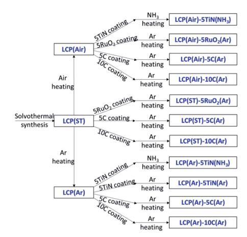
Scheme 2 Preparation conditions and sample labels for TiN, RuO<sub>2</sub> or C coated LiCoPO<sub>4</sub> materials.
