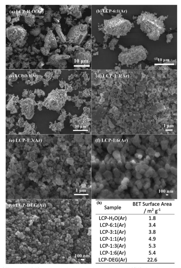
Fig. 1 (a-g) SEM images of LiCoPO<sub>4</sub> samples synthesised by the solvothermal method, using H<sub>2</sub>O/DEG solvent mixture with various volume ratios, followed by firing at 600 °C in Ar. (h) BET surface area of LiCoPO<sub>4</sub> samples.
