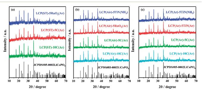
Fig. 5 XRD patterns of uncrystallised LiCoPO<sub>4</sub> directly after solvothermal synthesis (left), and LiCoPO<sub>4</sub> heated under air (centre) or Ar (right) at  $600 \,^{\circ}$ C, then modified with TiN, RuO<sub>2</sub> and carbon, respectively (labels explained in Scheme 2). The black stick pattern denotes the literature positions and intensities of LiCoPO<sub>4</sub> reflections.<sup>85</sup>
