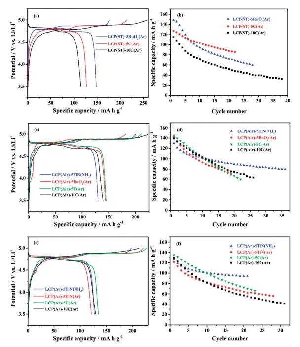
Fig. 6 (a), (c) and (e) The initial cycle voltage profile vs. specific capacity, and (b), (d) and (f) specific capacity vs. cycle number of TiN,  $RuO_2$  or C coated LiCoPO<sub>4</sub> samples made into Li half cells, under galvanostatic cycling between 3.5 and 5 V at 0.1C (sample labels explained in Scheme 2, with the percentage of TiN,  $RuO_2$  or C in the composite written after the hyphen).
