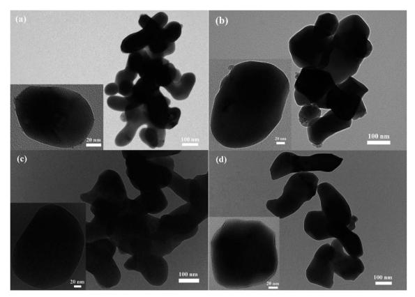
Fig. 3 TEM images of (a) LCP(Ar), (b) LCP(air), (c) LCP(H<sub>2</sub>N<sub>2</sub>) and (d) LCP(NH<sub>3</sub>) (scale bar = 100 nm). (Inset) magnified TEM images of single LiCoPO<sub>4</sub> particle (scale bar = 20 nm). Sample labels are explained in Scheme 1.
