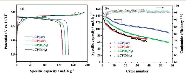
Fig. 4 (a) The initial cycle voltage profile vs. specific capacity and (b) specific capacity and coulombic efficiency vs. cycle number of LiCoPO<sub>4</sub>/Li half cells under galvanostatic cycling between 3.5 and 5 V at 0.1C (sample labels explained in Scheme 1).
