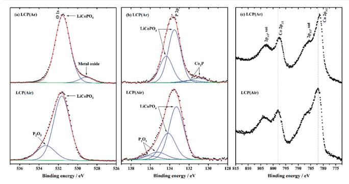
Fig. 8 P 2p, O 1s and Co 2p XPS spectra of LiCoPO<sub>4</sub> samples fired in Ar and air, respectively (labels explained in Scheme 1). The data points and enveloped fitting plot are overlaid in black dots and a red line, respectively. The fitting peaks and background are shown in blue and green, respectively.
